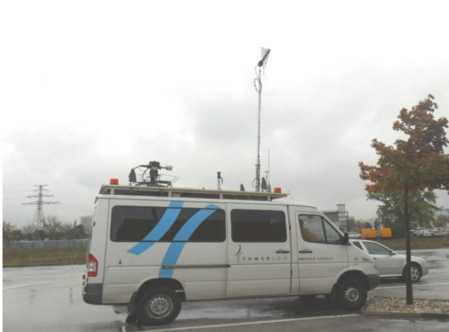
Figure 3 TOWERCOM's measurement van used in Bratislava city with a 5 m antenna height.
