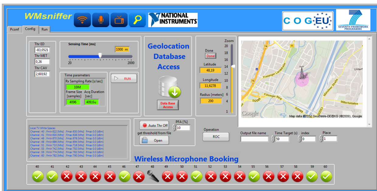
Figure 52: Setup interface for the COGEU sensing module: sensing time, threshold levels and the sensing algorithm are configuration parameters.
