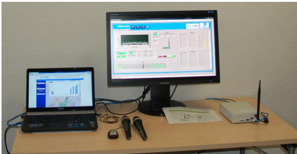
Figure 50: Photo of the deployed demonstrator, together with two wireless microphones. Both DVB-T geo-location database information (laptop screen) and PMSE sensing results (LCD screen) are displayed.
