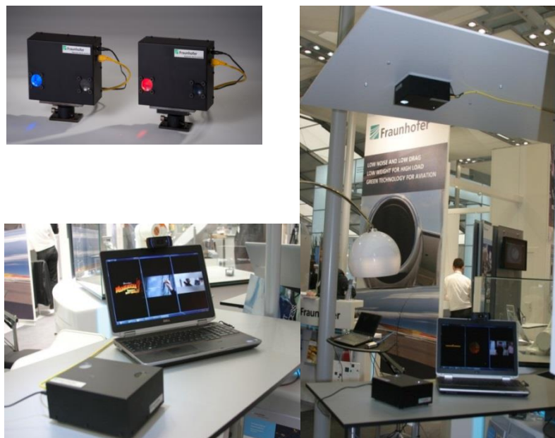
Figure 30: Real-time 500 Mb/s VLC system, as shown at a commercial exhibition (right) with the zoom-in of the desk part (bottom left) and the long-range (up to 20 m) version (top left).
