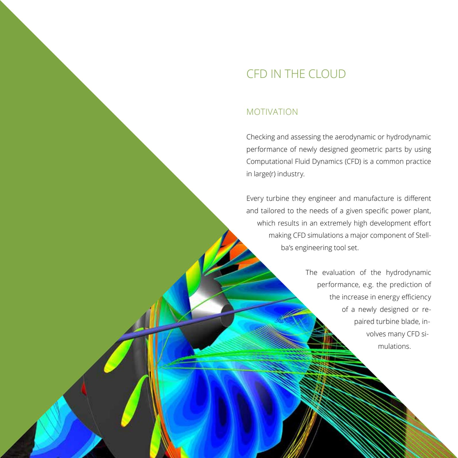
The full characterisation (hill chart) of a complex hydraulic turbine may require several hundreds of such simulations, where each simulation can take several hours to several days, depending on the available computing resources. Such a complete calculation is time and cost prohibitive when using traditional desktop machines.
