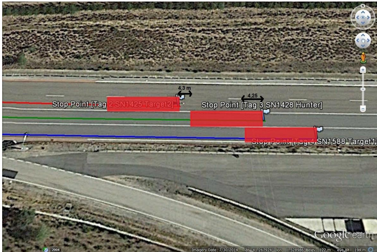
Figure 27. Gap between vehicles after emergency braking, 3 vehicles, 50 Km/h
