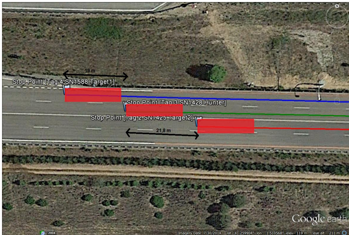
Figure 25. Gap after emergency braking of 3 vehicles at 50 Km/h
