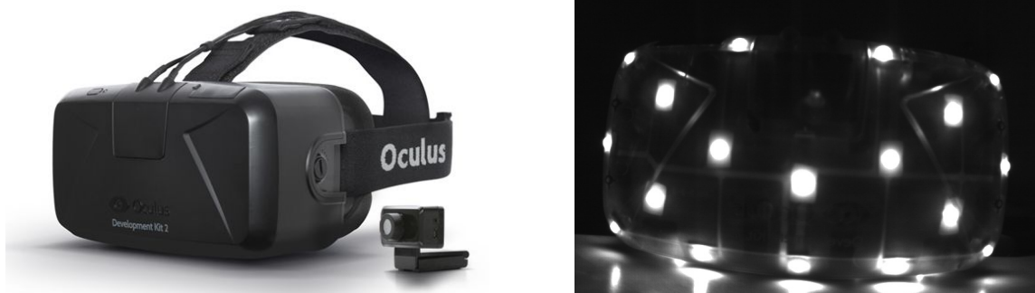
Figure 10: The Oculus Rift DK2 head-mounted display with the infrared sensor (left) and the front of DK2 with infrared LENSs active (right)
