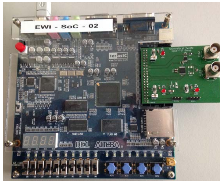
Figure 3.1-2: Actual implementation of the IRF generator. The FPGA houses the digital control, and the right-hand board the switches and resistors.
