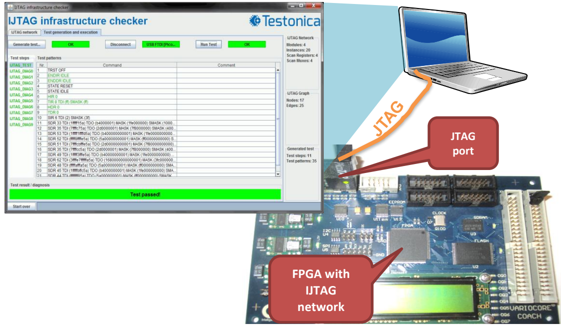
Figure 4. Experimental setup for IEEE 1687 IJTAG validator prototype
