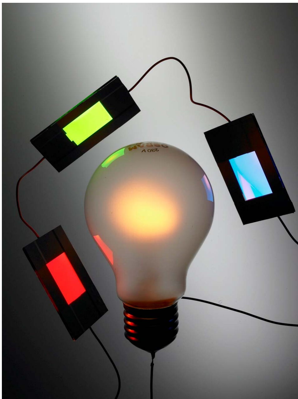
Caption: Colored small molecule OLEDs with Novaled PIN OLED™ technology for highest efficiencies and long lifetime devices. (Picture by Novaled)
