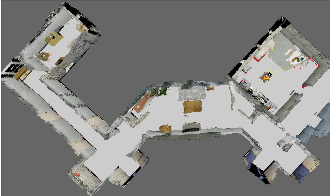
FIG. 41 THREE-DIMENSIONAL ENVIRONMENT MAP OF AN APARTMENT GENERATED FROM INFORMATION ACQUIRED BY THE ROBOT'S SENSORS WHILE DRIVING AROUND
