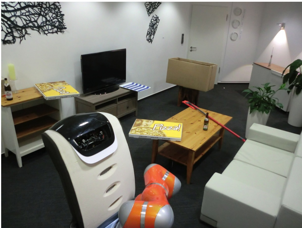
FIG. 50 ROBOT AT START FOR LIVING ROOM NAVIGATION TASK: USERS REMOTELY NAVIGATED THE ROBOT THROUGH SEVERAL OBSTACLES (PIZZA BOXES, DUST MOP, TRAY, CARTON)
