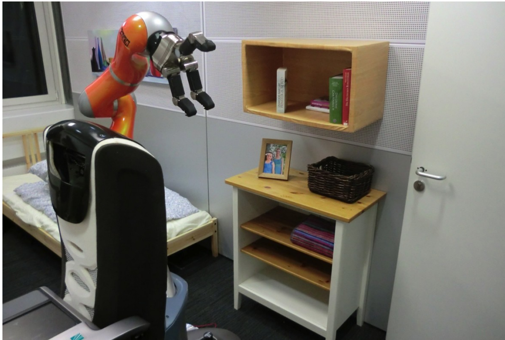
FIG. 51 ROBOT AT START FOR BEDROOM REMOTE MANIPULATION TASK: USERS REMOTELY NAVIGATED THE ARM TO THE LEFT BOOK AND THEN GRASPED IT. A TRAJECTORY OUT WAS THEN PERFORMED TO VERIFY THE GRASP.
