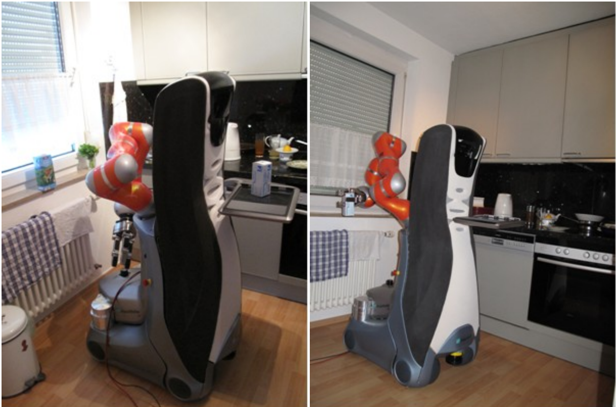
FIG. 15 MILK BOX (ON SILL IN THE LEFT PICTURE) AS A SUBSTITUTE OBJECT FOR MEDICINE BOX (ON SILL IN THE RIGHT PICTURE) TO CIRCUMVENT TEACHING OF MEDICINE BOX; USAGE OF ARTIFICIAL LIGHT TO ENABLE OBJECT DETECTION BECAUSE OF BACKLIGHT ENTERING THROUGH WINDOW
