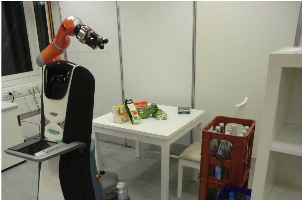
FIG. 48 ROBOT AT START FOR KITCHEN REMOTE MANIPULATION TASK: USERS REMOTELY NAVIGATED THE ARM TO THE APPLE JUICE BOX AND THEN GRASPED IT. A TRAJECTORY OUT WAS THEN PERFORMED TO VERIFY THE GRASP.
