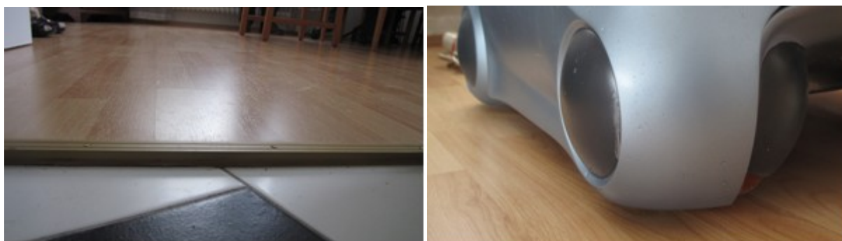
FIG. 17 PROBLEMATIC DOOR SILL (LEFT); LOWER BOUND OF ROBOT SHELL (RIGHT)
