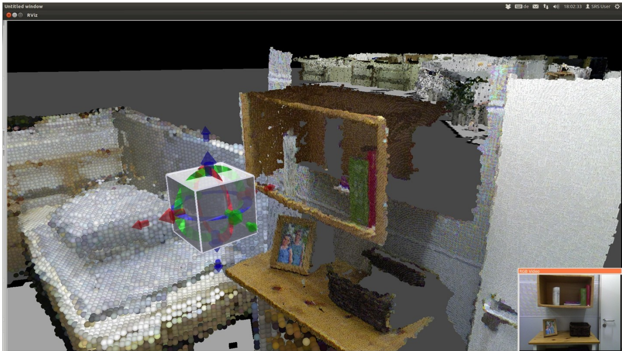
FIG. 44 REMOTE SEMI-AUTONOMOUS MANIPULATION STEP 1: USER SPECIFIES SIZE, POSITION, AND ORIENTATION OF BOUNDING BOX (BOX IS PLACED OVER THE TARGET OBJECT, IN THIS CASE A BOOK IN A SHELF)
