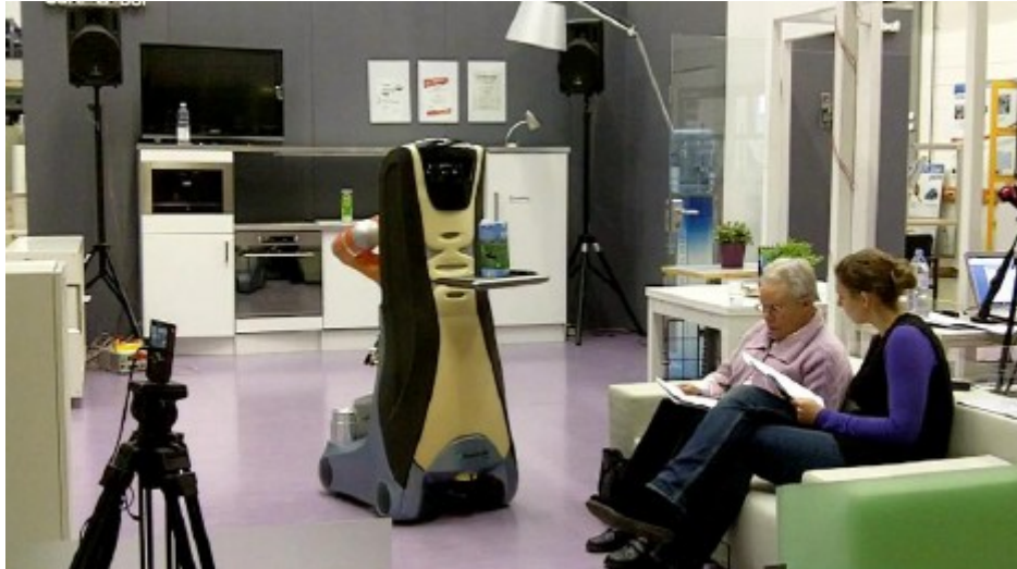
Figure 9: Robot got milk for the elderly based on the request sent from the smart phone (UI_LOC)
