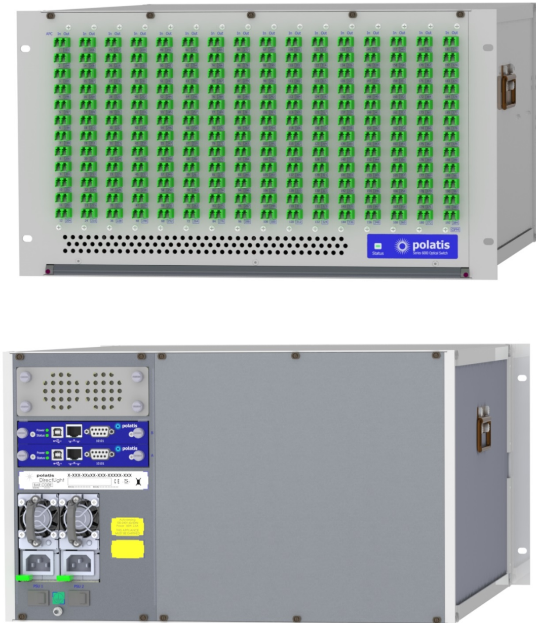
Figure 2 A standard Polatis 192x192 optical circuit switch with LC/APC connectors: front panel(above); rear panel (below) showing redundant hot-swappable network interface cards, power supply units and fans
