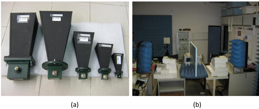
FIGURE 40. Measurement of foam characteristics; (a) Standard horns; (b) Measurement setup.
