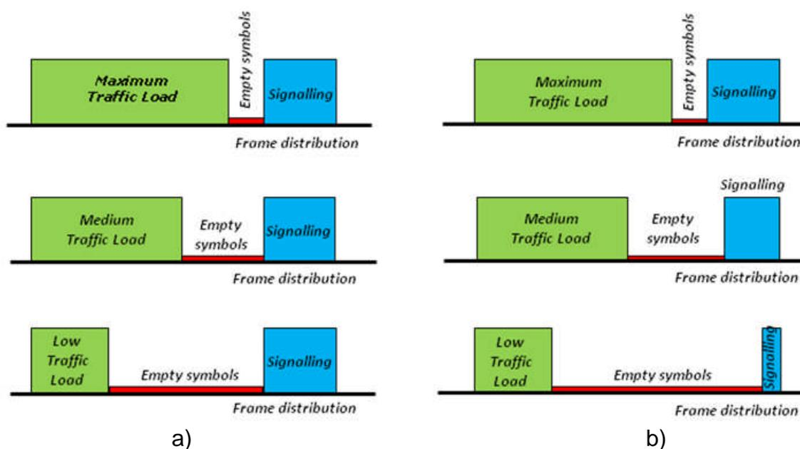
Figure 30 Different LTE frame distributions according to the traffic load a) without cell DTX and b) with cell DTX
