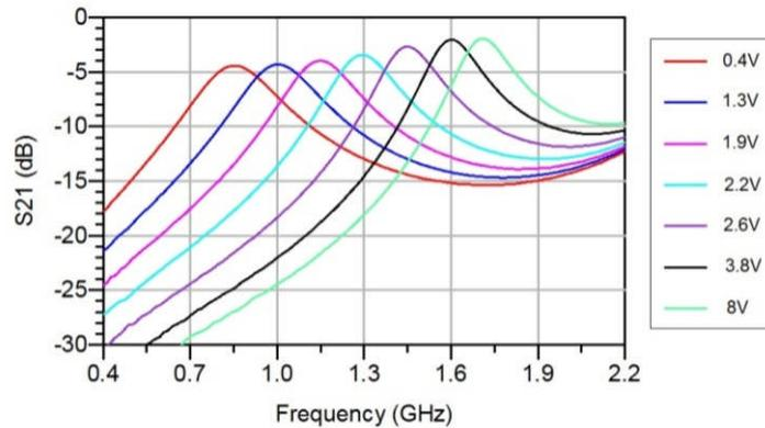
**Figure 28 a) Measured insertion loss of the varactor-tunable SIR**
