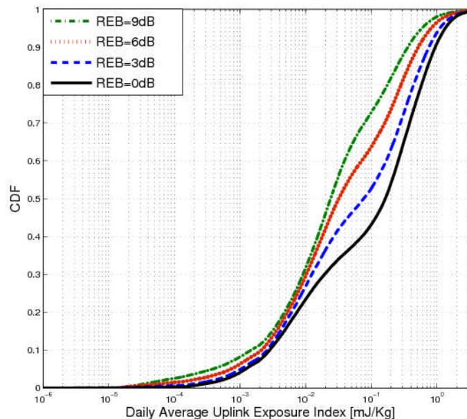
**Figure 23 Cumulative distribution functions of the daily average UL EI at UEs for different REB values.**
