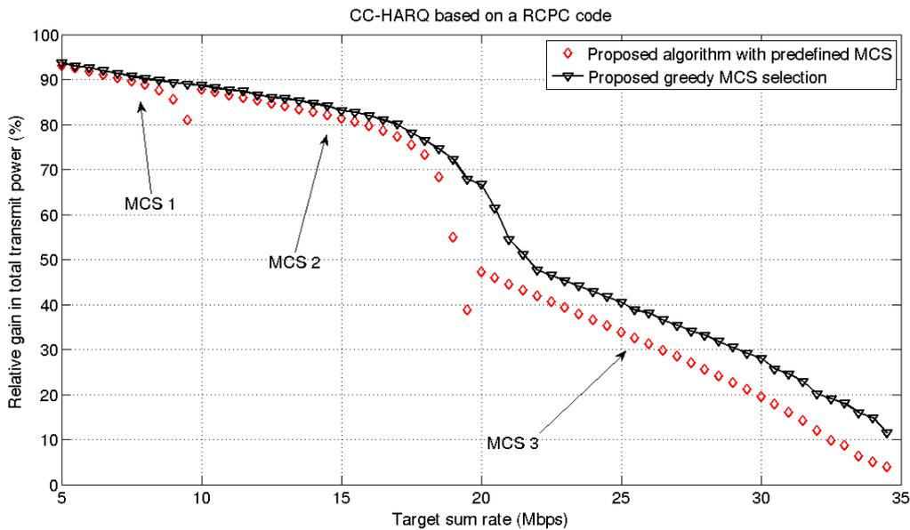
**Figure 55 Sum transmit power gain vs. Sum target rate for the proposed algorithms when CC-HARQ is implemented**
