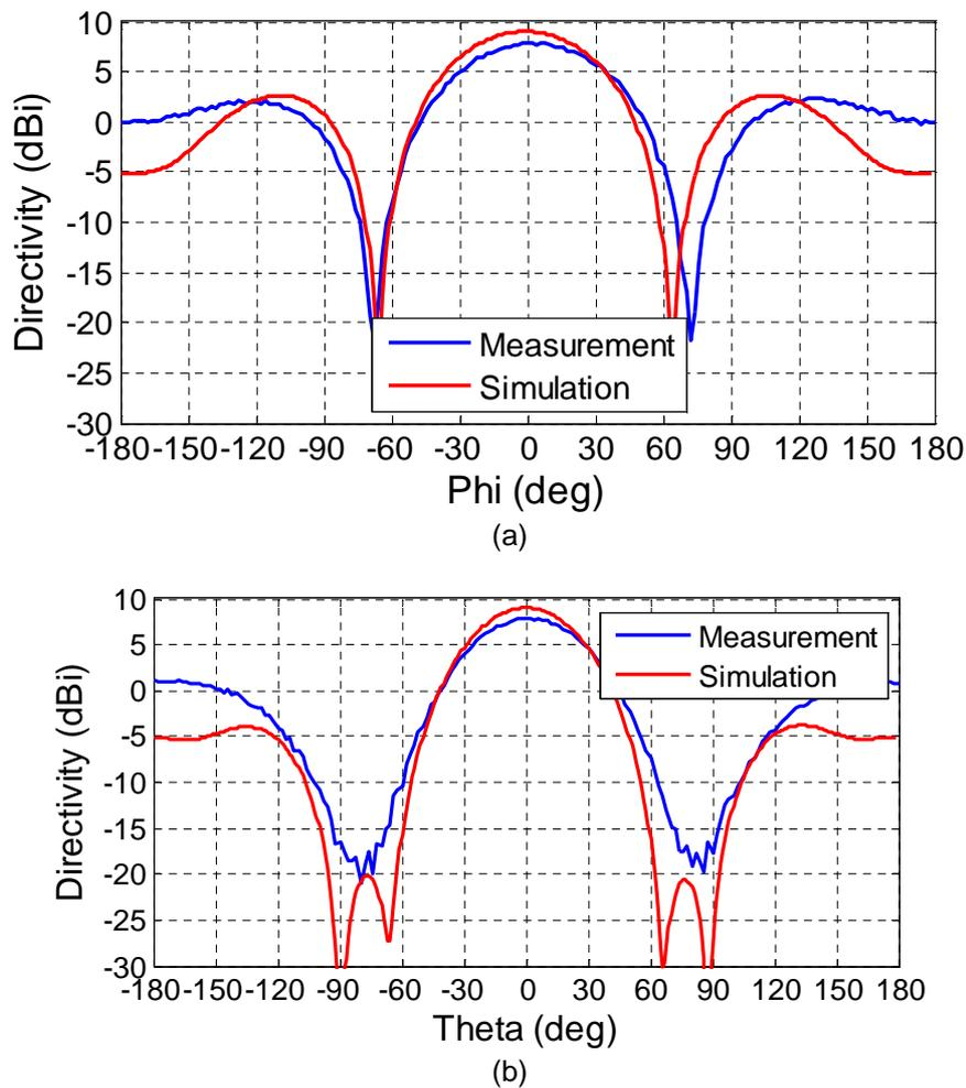
**Figure 19 Measured and simulated directivity radiation pattern (simulation frequency 868 MHz, measurement frequency 872) of the three-element computed on the (a) H- and (b) E-plane.**
