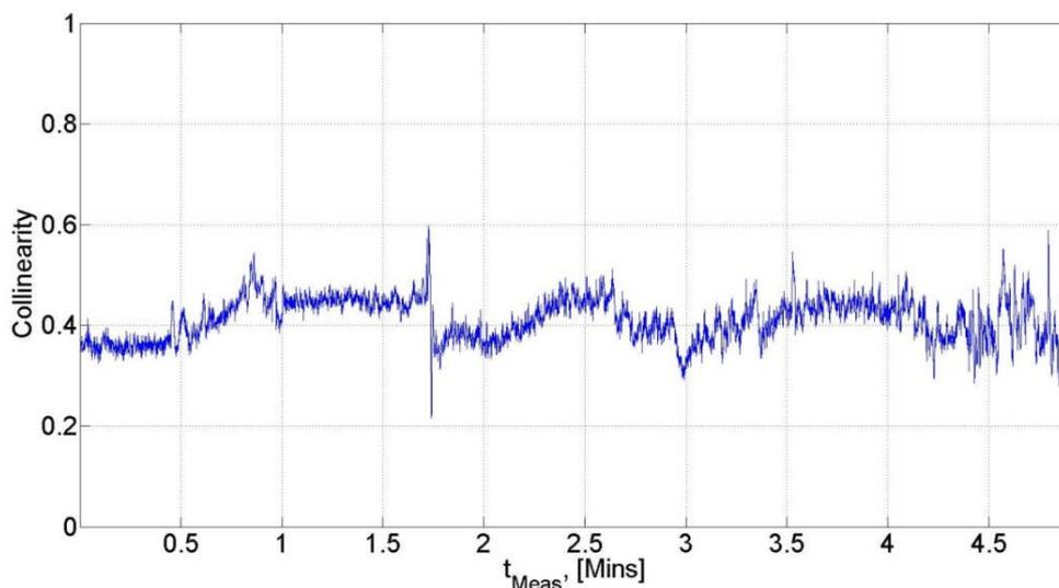
**Figure 11: Collinearity of channels: laptop-probes and laptop-access point over time,  $t_{Meas}$ .**
