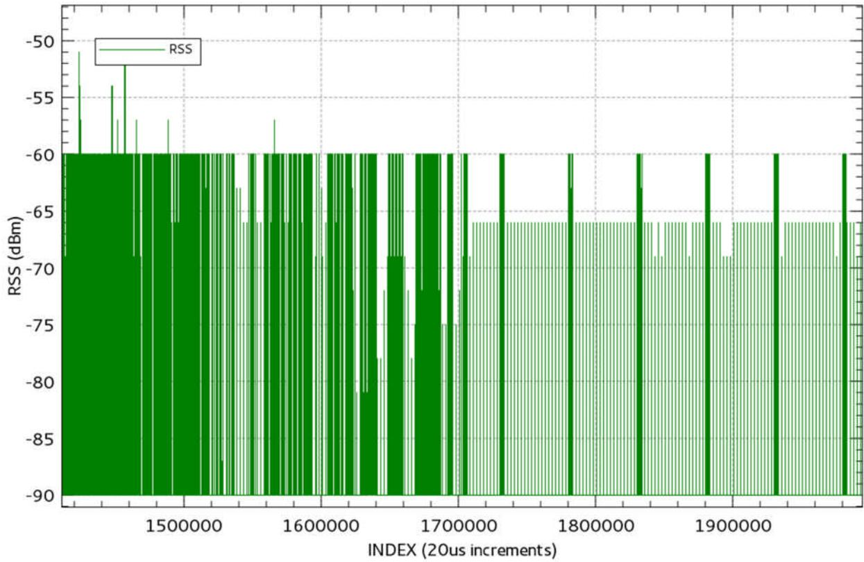
Figure 46 Moment of interference between ZigBee and Wi-Fi
