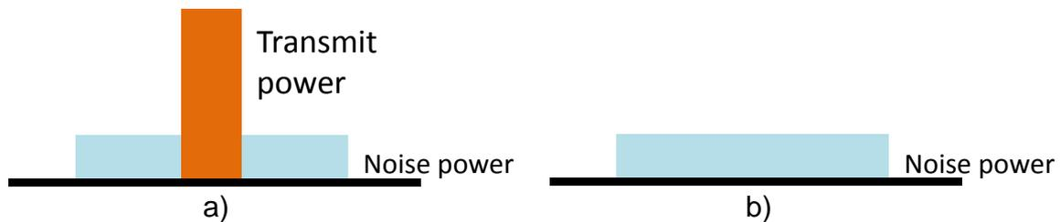
Figure 31 RF spectrum for a) non empty symbols and b) empty symbols without a specific HPA to implement cell DTX
