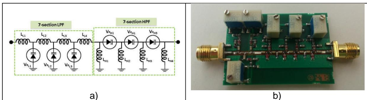
**Figure 25 a) Electrical diagram of reconfigurable BPF (7-section LPF and 7-section HPF) based on varactors and b) Manufactured prototype**
