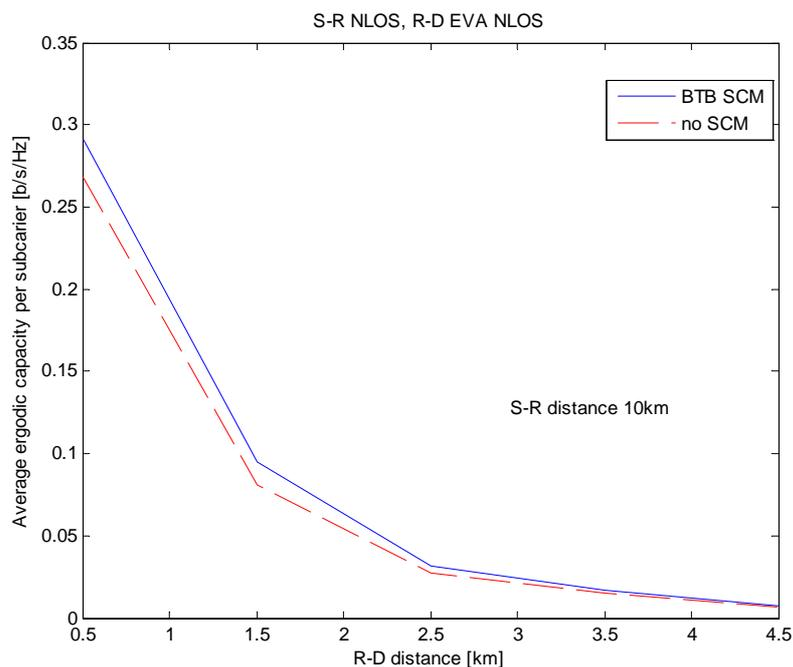
**Figure 53 Average ergodic capacity per subcarrier for OFDM DF systems with BTB SCM and no SCM (S-R NLOS, R-D EVA NLOS scenario)**
