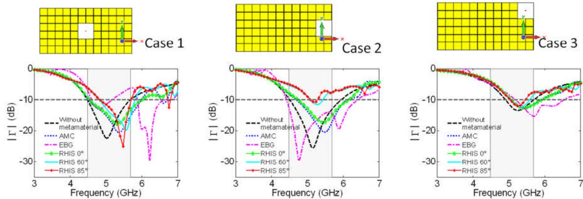
**Figure 62 Impedance matching.** Case 1: antenna at centre. Case 2: antenna at middle of the edge. Case 3: antenna on the corner
