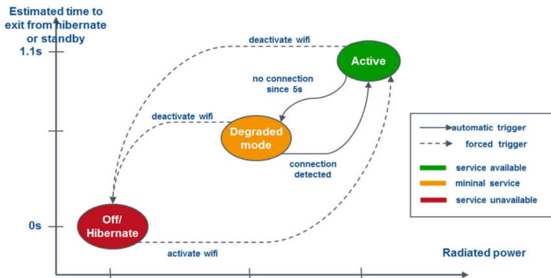
Figure 32 Idle-enabled State-Machine of a WLAN Access Point
