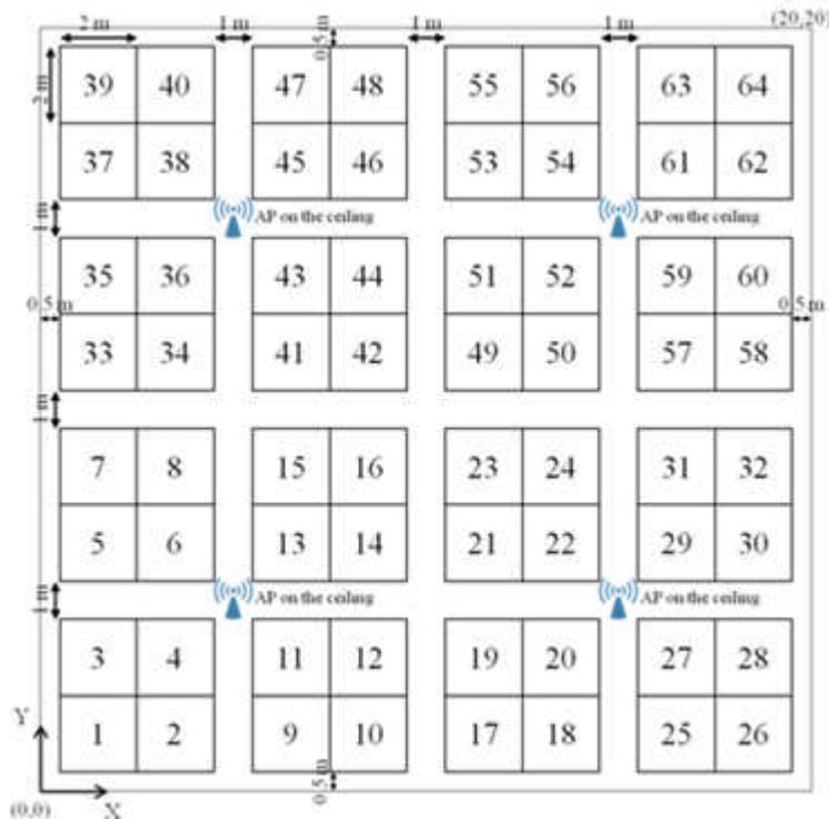
Figure 34 IEEE 802.11 enterprise layout for a single BSS [43]
