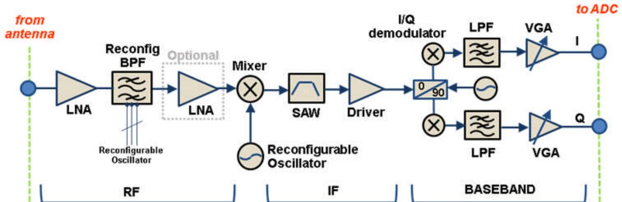
Figure 24 Proposed block diagram for reconfigurable low noise receiver
