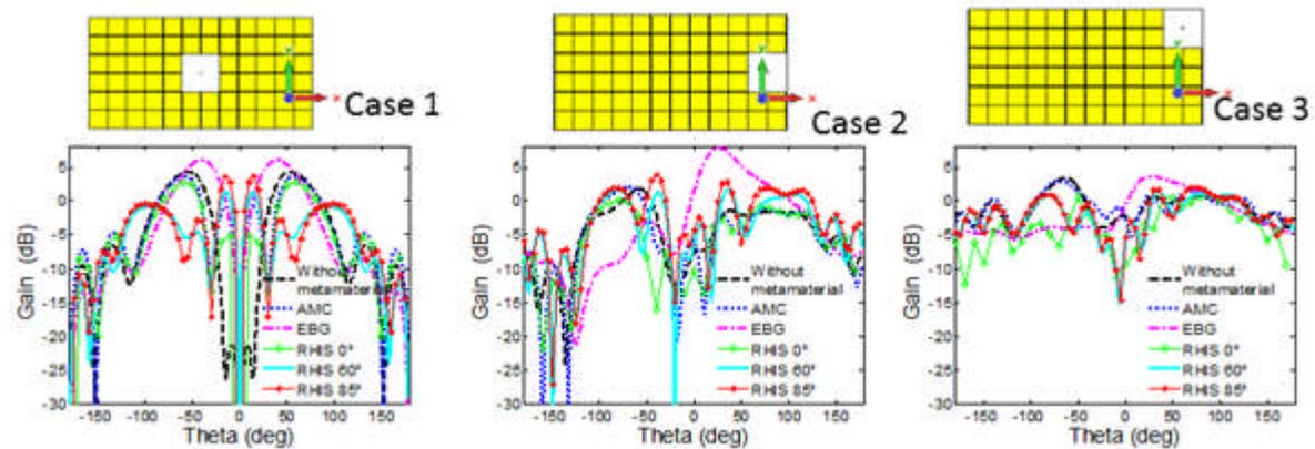
Figure 65 Gain Radiation pattern. Plane  $\phi = 0^\circ$ . Case 1: antenna at centre. Case 2: antenna at middle of the edge. Case 3: antenna on the corner
