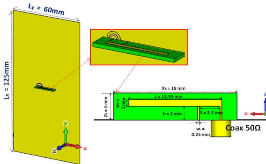
Figure 58 IFA Antenna configuration
