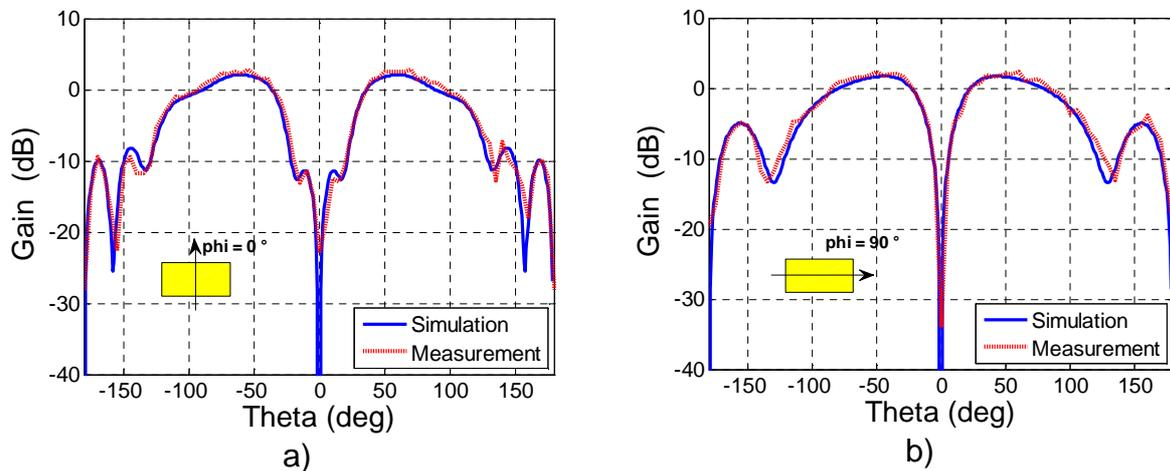
Figure 78 Gain, monopole antenna without metamaterial. a) Plan  $\phi = 0^\circ$ . b) Plan  $\phi = 90^\circ$ .
