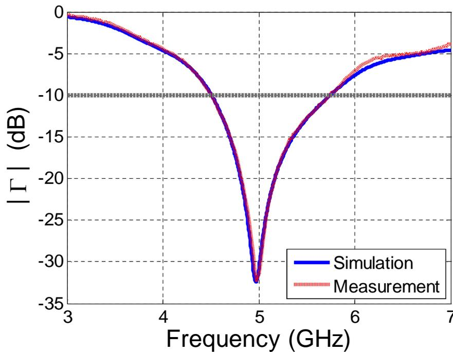
Figure 76 Impedance matching monopole antenna without metamaterial
