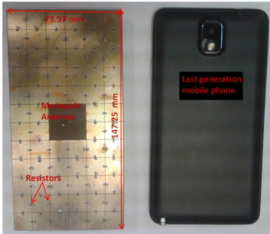
Figure 75 Monopole antenna with RHIS structure
