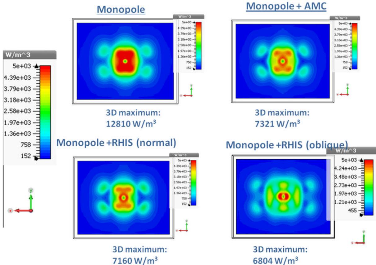
Figure 6 Power loss density, spatial distribution, Monopole Antenna
