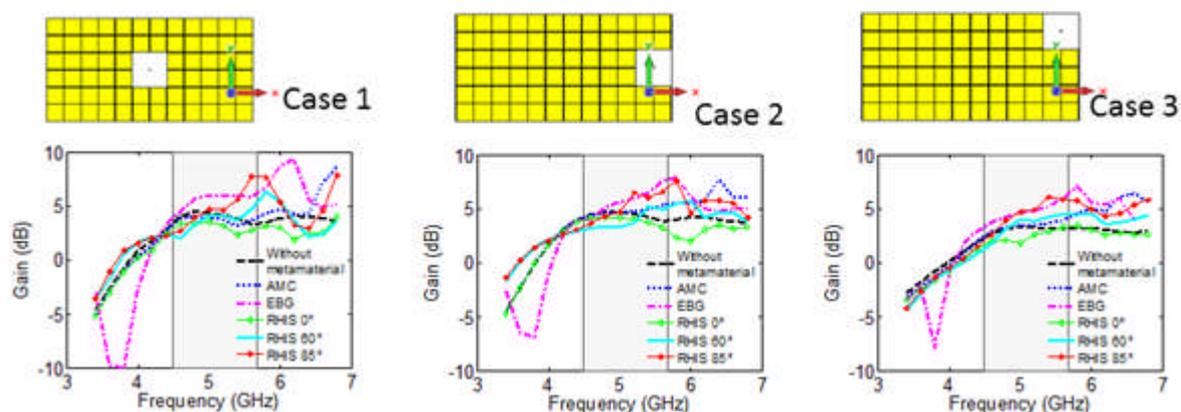
**Figure 64 Realised Gain.** Case 1: antenna at centre. Case 2: antenna at middle of the edge. Case 3: antenna on the corner
