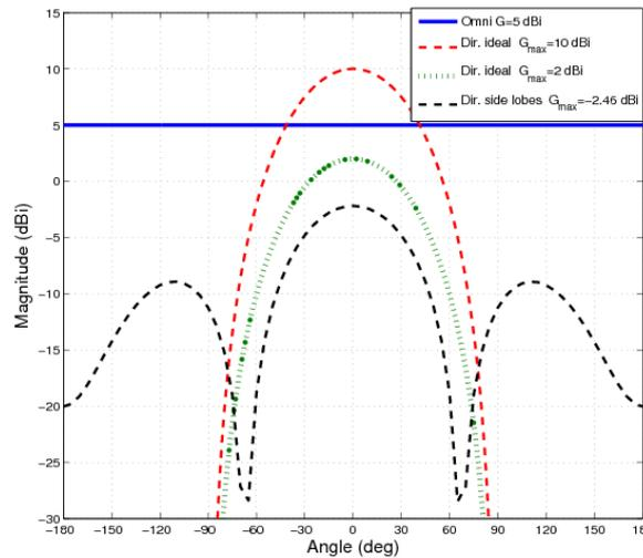
Figure 21. Gain radiation patterns of the antenna models used in the numerical analysis.
