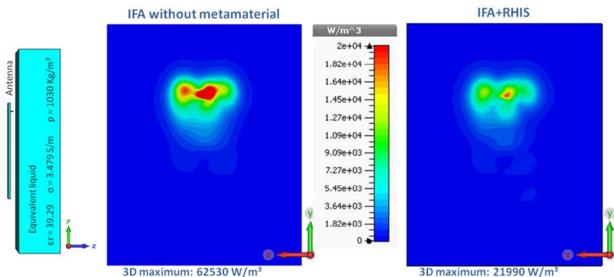
Figure 8 Power loss density, spatial distribution, IFA Antenna
