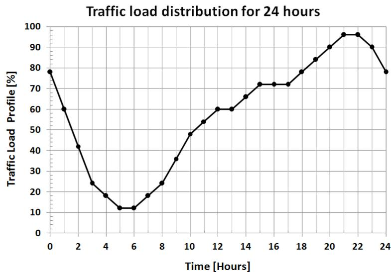
Figure 29 24 hours traffic load profile – Urban area during a day [38]
