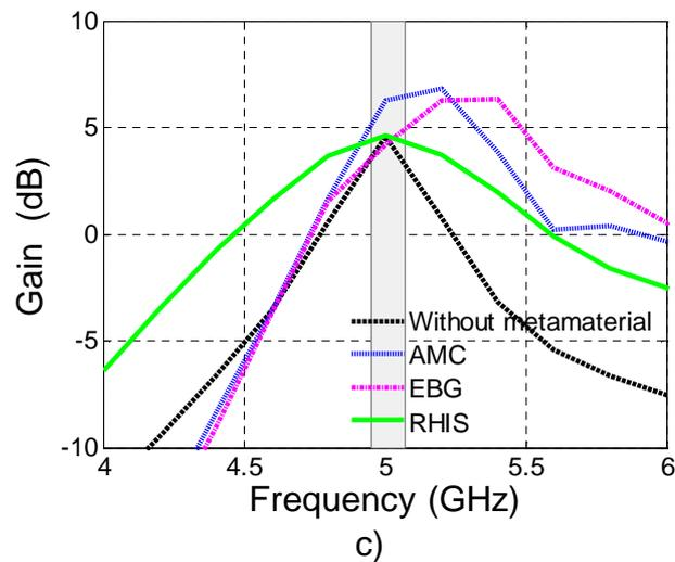
Figure 7 QoS KPI IFA Antenna a) Antenna matching b) Total efficiency c) Gain
