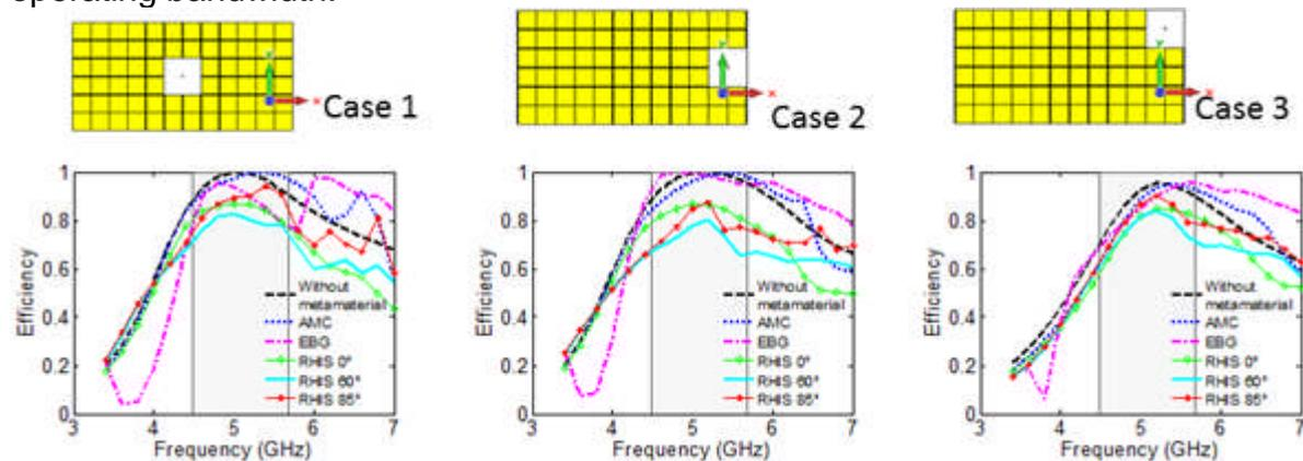
**Figure 63 Efficiency.** Case 1: antenna at centre. Case 2: antenna at middle of the edge. Case 3: antenna on the corner
