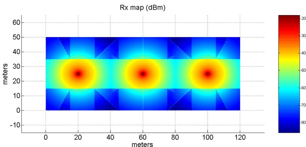
Figure 39 Received power map with all APs running in SISO idle mode (2.4GHz only)
