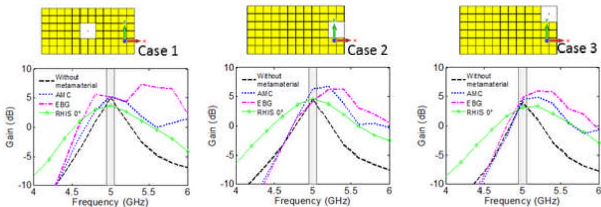
Figure 70 Realised Gain. Case 1: antenna at centre. Case 2: antenna at middle of the edge. Case 3: antenna on the corner
