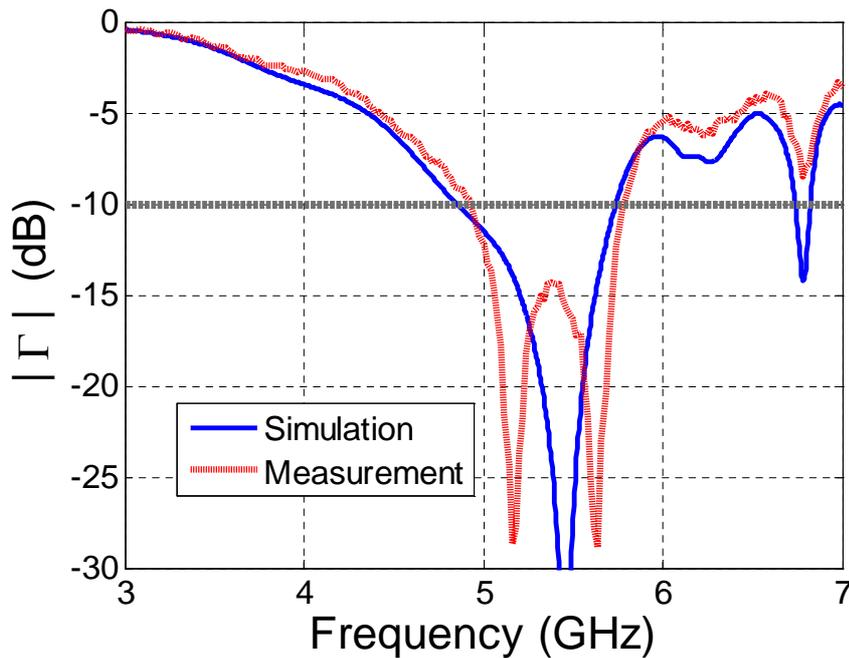
Figure 77 Impedance matching monopole antenna with RHIS
