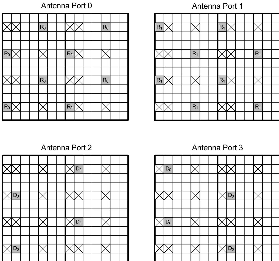
Figure 43 A new DMRS pattern configured on 2 CRS antenna ports in the 4 CRS ports case
