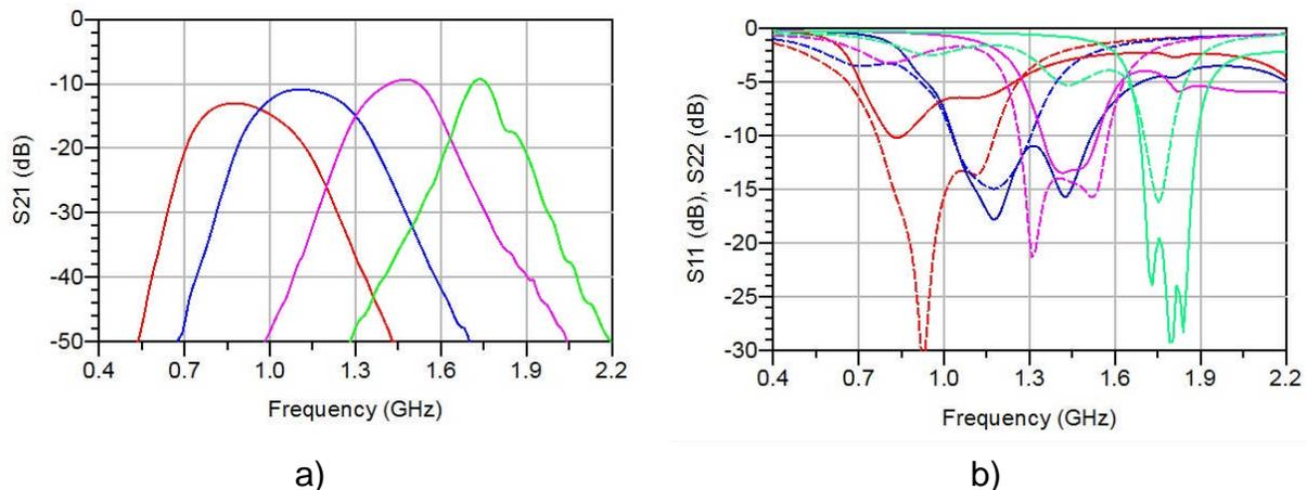
**Figure 26 a) Measured insertion loss and b) Measured return losses of reconfigurable BPF (7-section LPF and 7-section HPF) based on varactors**
