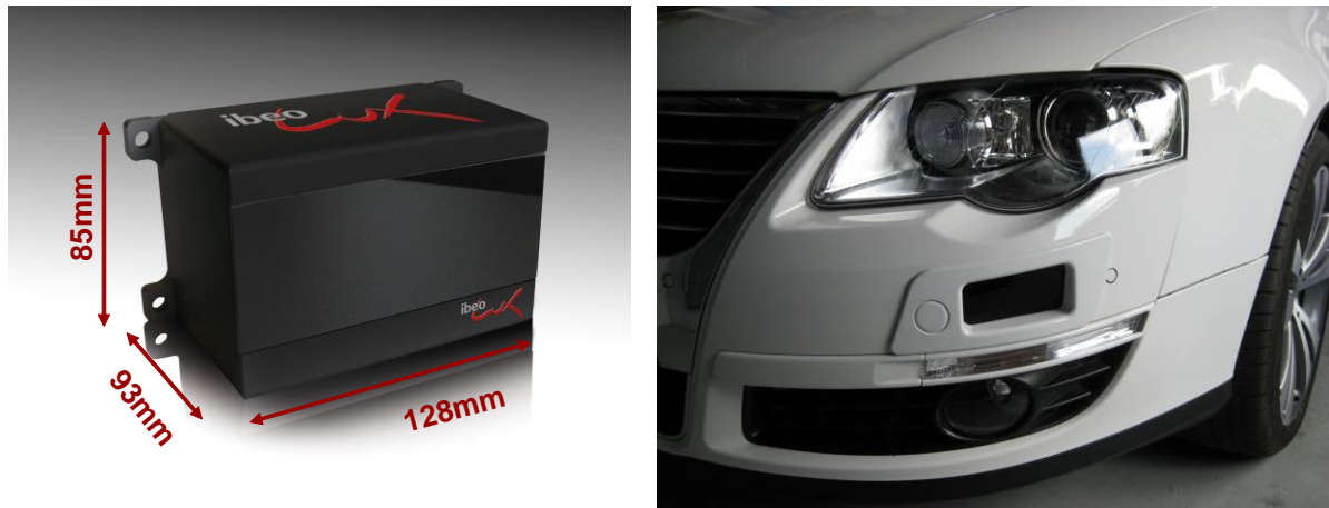
Figure 143: Laser scanner component and its final position mounted below the beams
