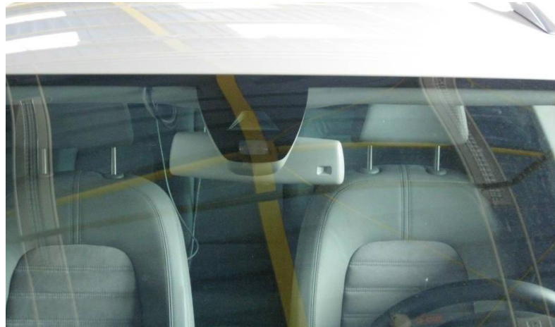
Figure 144: Location of the lane detection camera mounted above the rear mirror
