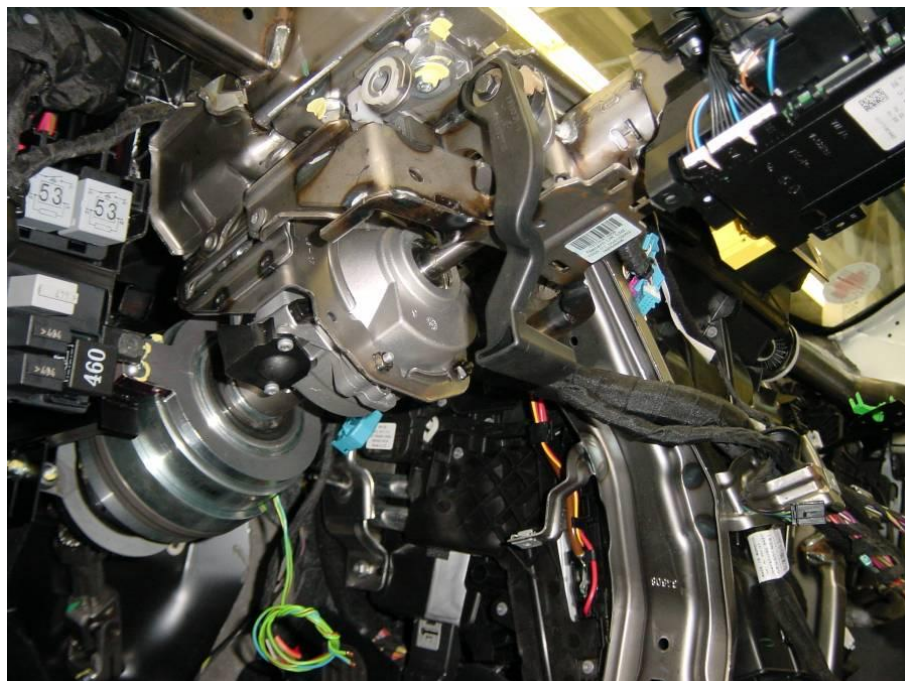
Figure 63: Steering column (clutch and feedback actuator) integrated in the vehicle
