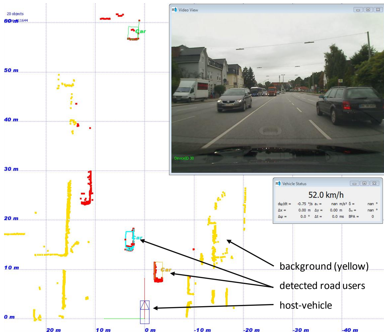
Figure 72: Tracked and classified road users, based on laser scanner data
