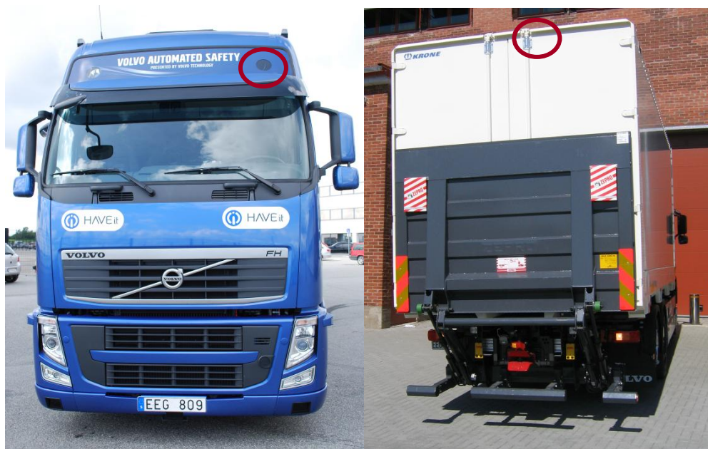
Figure 39: Integration of the V2V units on the AQuA truck.
