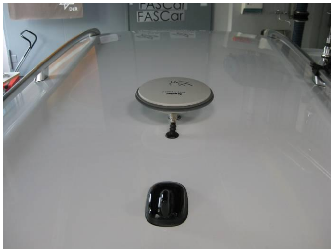
Figure 145: GPS receiver antenna mounted on the roof of the vehicle
