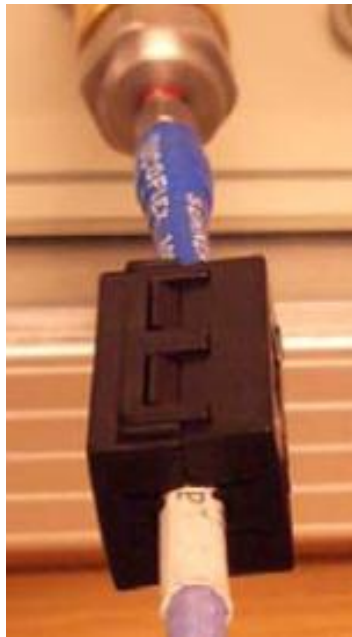
Figure 7.4.3 Use of ferrite to reduce leakage current
