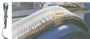
Integration of the sensor textile in c leg of a sports prosthesis
