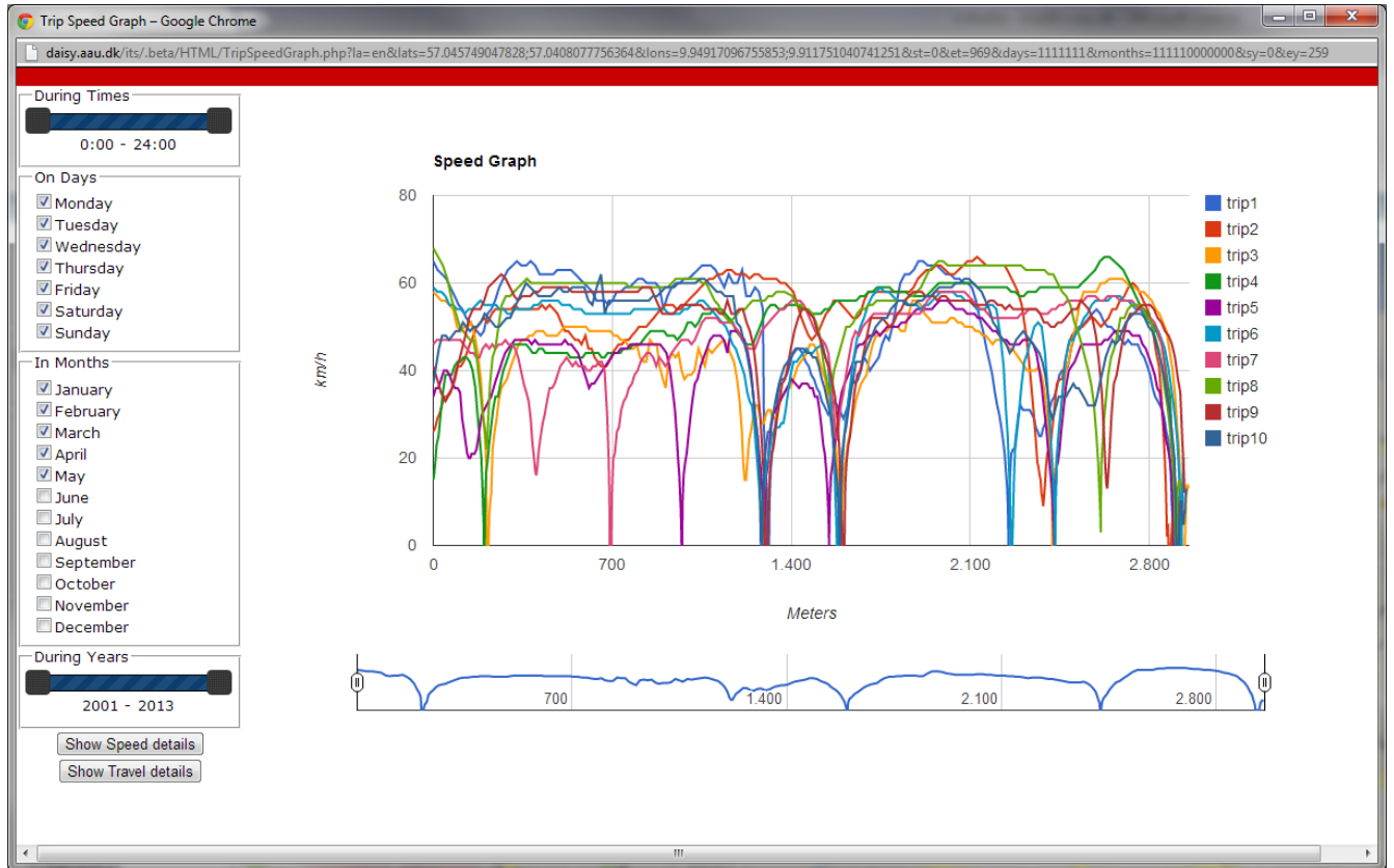
Figure 19: Using High-Frequent GNSS Data to Identify Intersections
