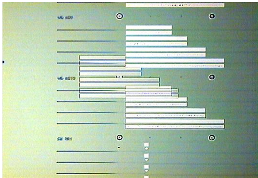
Figure 7.2: Test chip of the integrated Si-implanted photodiodes.
