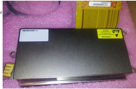
Figure 2.1 – Left: Finisar WSS design, employing free-space optics and an LCoS switching engine. Right: FOX-C prototype WSS offering 20 output fibre ports, flex-grid operation, and 7.5 GHz optical resolution.
