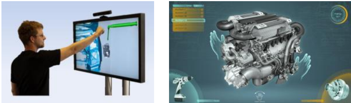
Figure 1: Interaction Concept for Virtual Assembly Training
