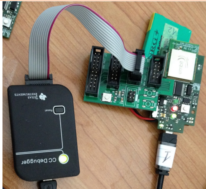
Figure 4-16: Representation EMB-Z2530PA sensor with debugger.
