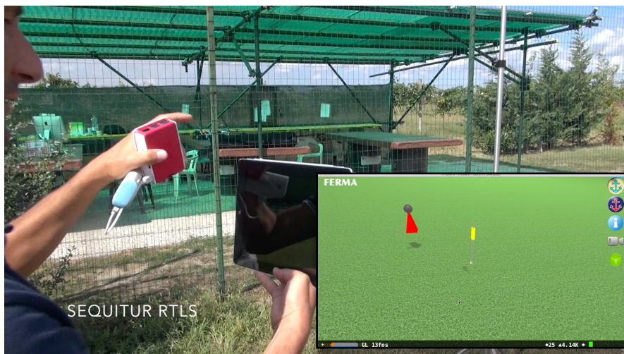
Figure 4-6: Tracking of humans using UWB signals
