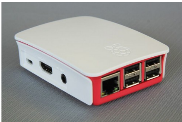
Figure 4-1 The Raspberry Pi 2 micro-PC adopted as anchor nodes.
