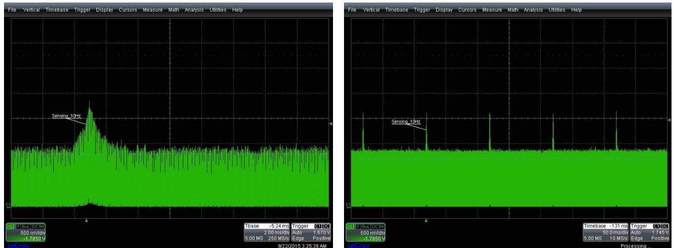
Figure 44: Current waveforms during conversion: one and four conversion cycles
