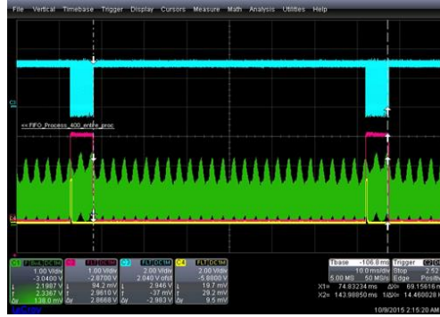
Figure 57: ODR 400Hz watermark 24, FIFO mode and reading period
