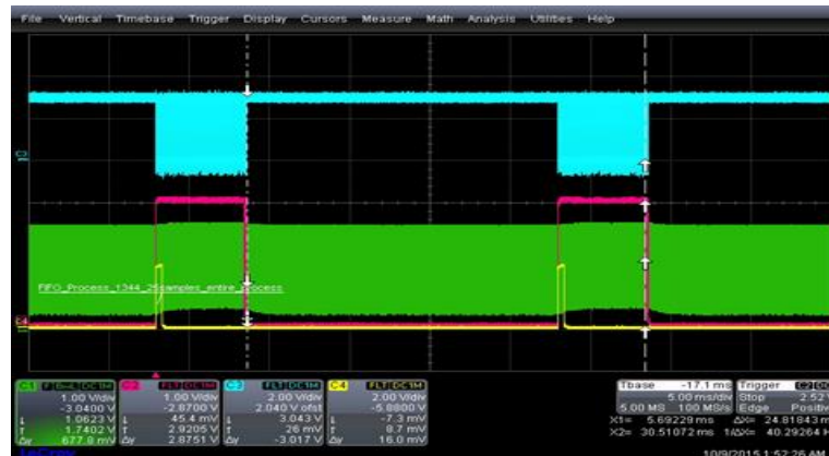
Figure 55: ODR 1344Hz watermark 25, FIFO mode and reading period
