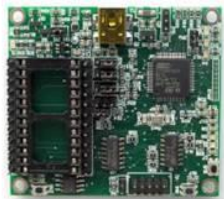
Figure 34: STEVAL-MKI109V2 evaluation board
