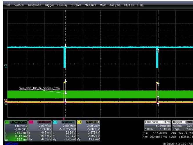
Figure 68: ODR 100Hz, watermark 24, FIFO mode and reading period
