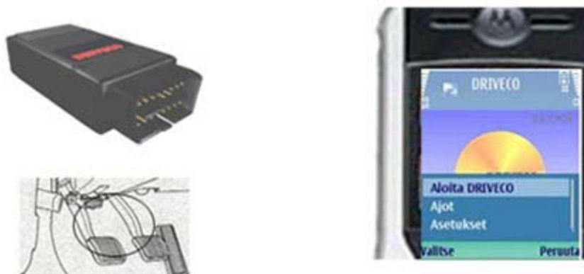
Figure 8: DRIVECO OBD-II module and mobile phone application.
