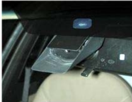
Figure 57: The Lane Departure Camera
