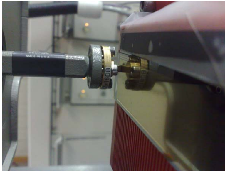
Fig. 18 Photograph of the setup of the S_{11} measurement.
