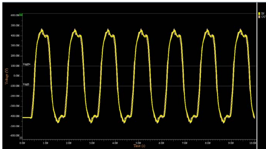
Figure 5.1-5 Signal integrity simulation including test board and custom lead frame. Signal reaching the integrated DAC LVDS pads from FMC connector
