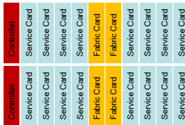
Figure 3-10: architecture of the DISCUS MPLS-TP core switch.
