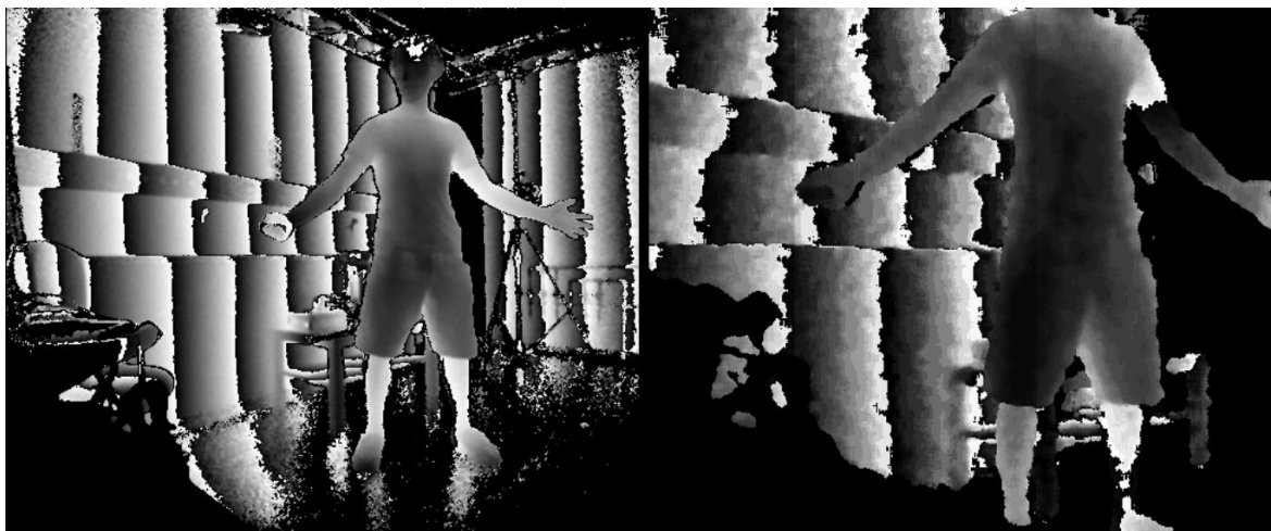
Figure 3.2: Kinect 2 (left) vs. Kinect 1 (right) depth image
