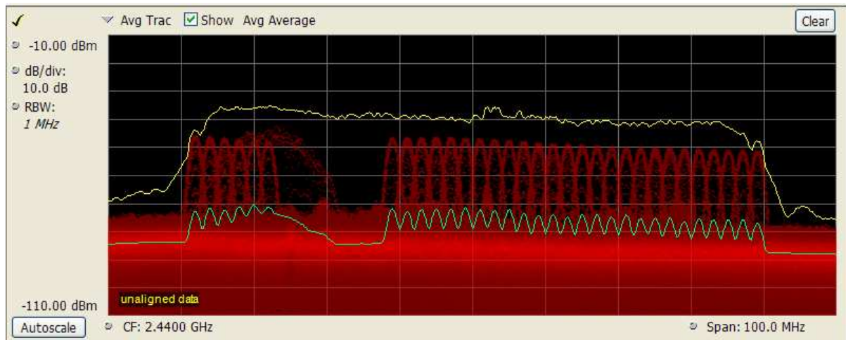
Fig. 30: DPX spectrum of the WISMIT signals at center frequency of 2.442 GHz together with Bluetooth signals in several bands (max. hold: yellow, average: green).
