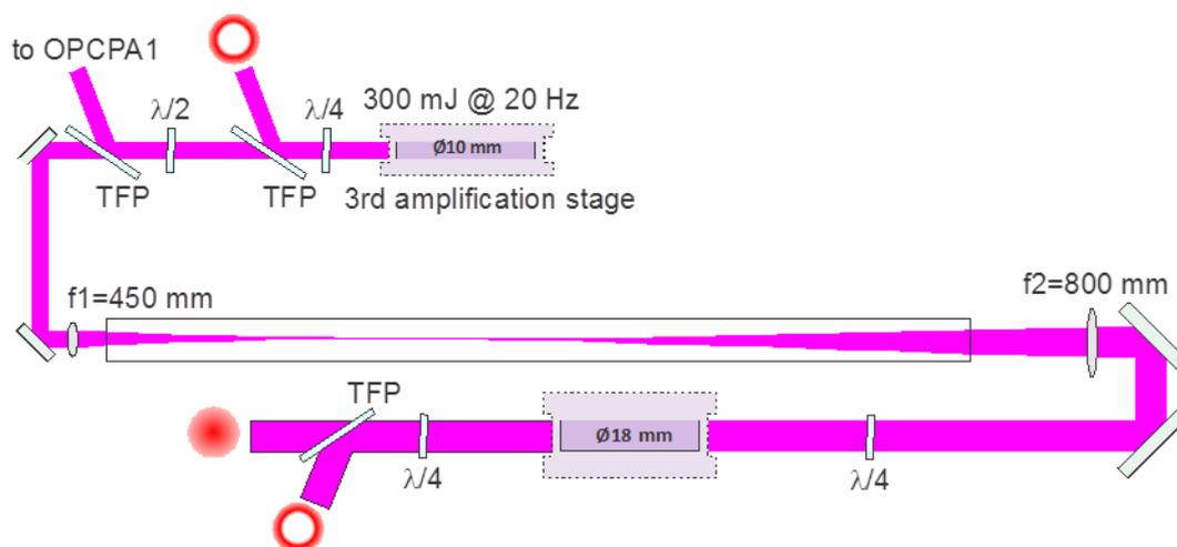
*Fig. 1. Experimental arrangement of the last amplification stage. The input of the last amplification stage is provided by the output of the previous amplification stage, after the splitting of a portion of energy for the pumping of the first OPCPA1 stage. TFP are thin film polarizers,  $\lambda/2$  and  $\lambda/4$  are half and quarter wavelength retardation plates, respectively.*
