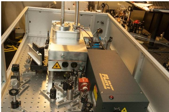
*Fig. 8. Left: Femtosecond CPA and OPA at TU Wien before shipment to MSU. Right: zoom on the oscillator built by Light Conversion and the regenerative amplifier developed at TU Wien.*
