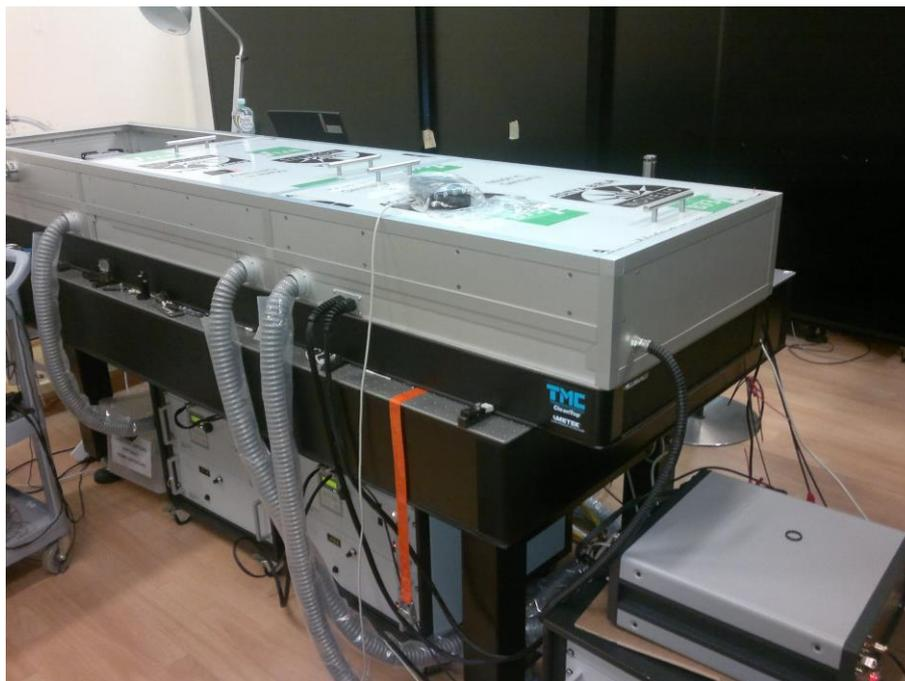
*Fig. 7. 3-Channel 20-Hz 100-ps pump laser built by EKSPLA*
