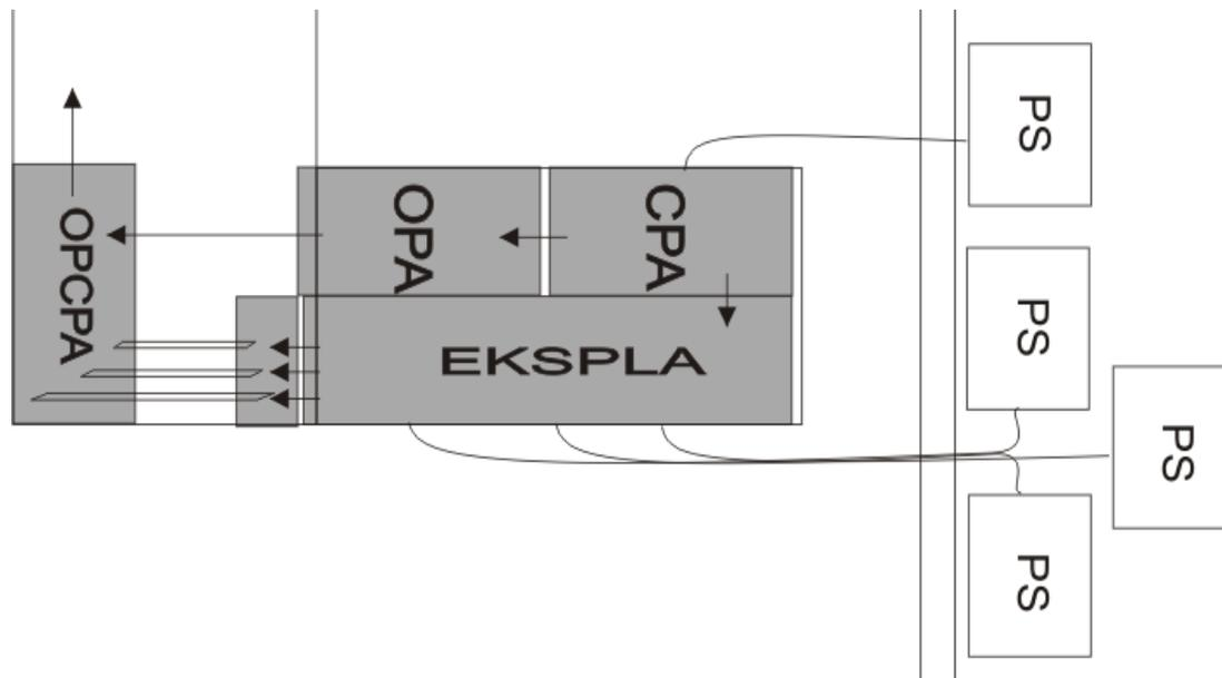
Fig. 6. Layout of the high-energy 20-Hz MID-IR OPCPA to be installed in Moscow. PS, power supply
