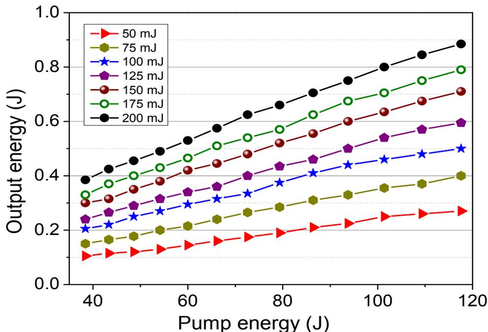
Fig.3. Dependence of the output energy of the last amplification stage on pump energy at different seed pulse energy (indicated in the figure).
