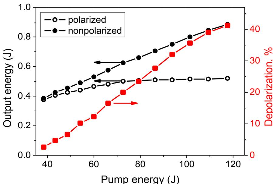
Fig.5. Dependence of the total output energy (left ordinate axis, solid black circles) and energy contained in the p-polarized pulse (left ordinate axis, open black circles); by the red squares the percentage ratio of depolarized light (right ordinate axis), which is separated by the TFP and possess donut-structure (Fig.1) is presented.
