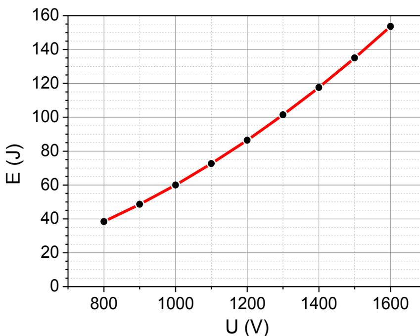
*Fig. 2. The dependence of pump pulse energy on the output voltage of the dual power supply.*
