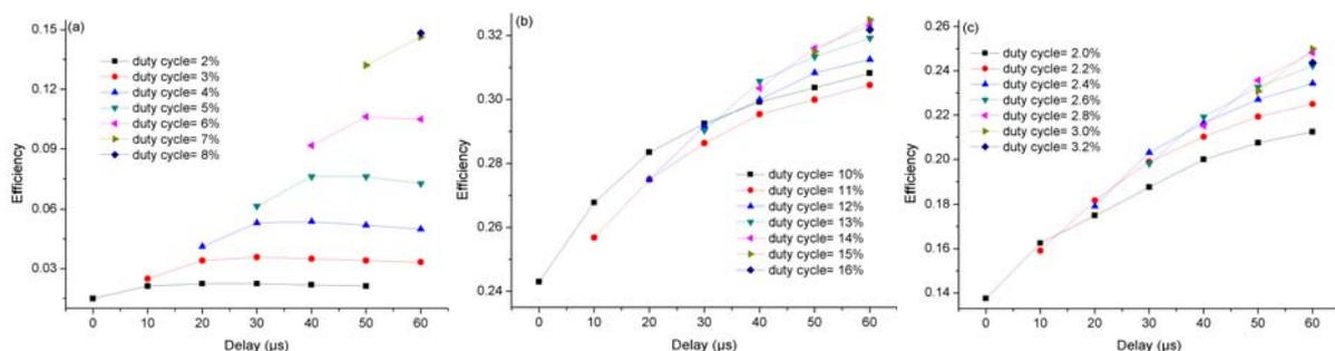
Fig. 5. Pump-to-signal conversion efficiency for pulse burst lengths of (a) 20  $\mu$ s, (b) 100  $\mu$ s at 1 kHz and (c) 100  $\mu$ s at 200 Hz as a function of the delay between the rising edges of the pump and signal emissions for various pump duty cycles. The lines are only to guide the eye.
