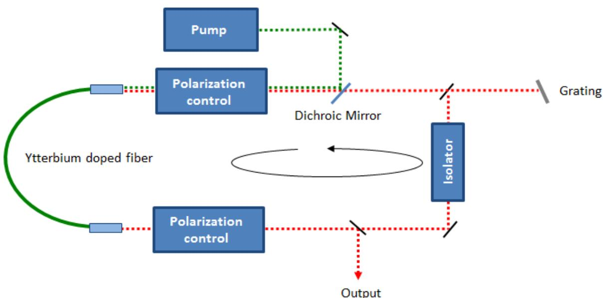
Fig. 1. All-normal dispersive setup of the oscillator. An isolating unit is stipulating the direction of the propagating laser light. A grating with 300 lines/mm assists the modelocking mechanism. The pump light is coupled into the laser ring via a dichroic mirror.
