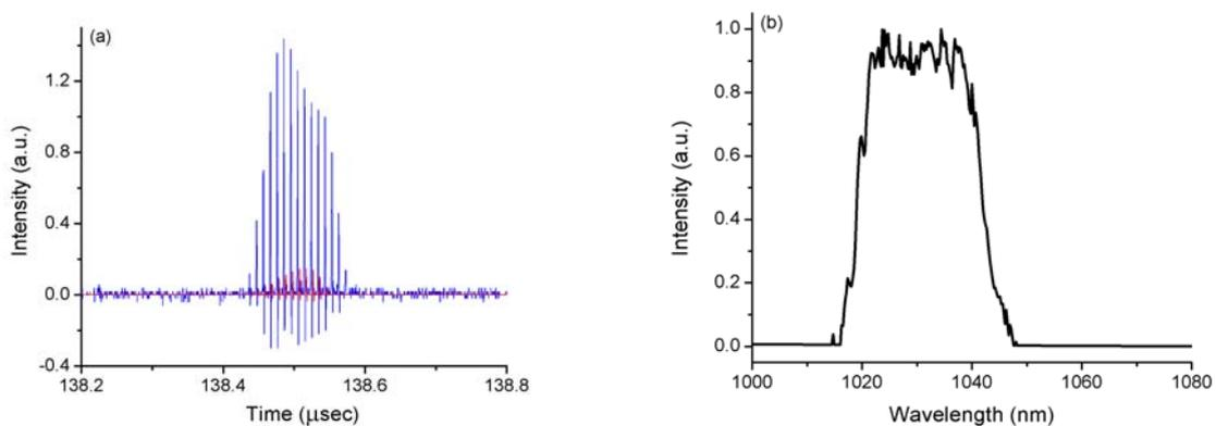
Fig. 11. (a) Output (blue line) and Input (red line) pulse train, (b) output spectrum for 150 ns signal burst, output power of 270 mW, average output pulse energy of 17.3  $\mu\text{J}$ , highest pulse energy of 27  $\mu\text{J}$ .
