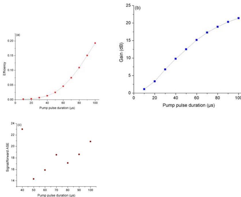
Fig. 9. The measured (a) pump-to-signal conversion efficiency, (b) signal gain factor and (c) ASE formation as a function of pump pulse duration for a 1- $\mu\text{s}$  signal burst at a repetition rate of 1 kHz. The lines are only to guide the eye.
