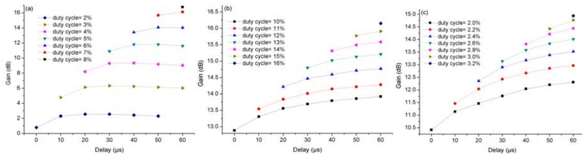
Fig. 7. The measured signal gain ratios for pulse burst lengths of (a) 20  $\mu\text{s}$ , (b) 100  $\mu\text{s}$  at 1 kHz and (c) 100  $\mu\text{s}$  at 200 Hz as a function of the delay between the rising edges of the pump and signal emissions for various pump duty cycles. The lines are only to guide the eye.
