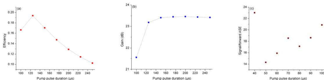
Fig. 10. The measured (a) pump-to-signal conversion efficiency, (b) signal gain factor and (c) ASE formation vs. pump pulse duration from 100 to 250  $\mu$ s for a 1- $\mu$ s signal burst at a repetition rate of 1 kHz. The lines are only to guide the eye.
