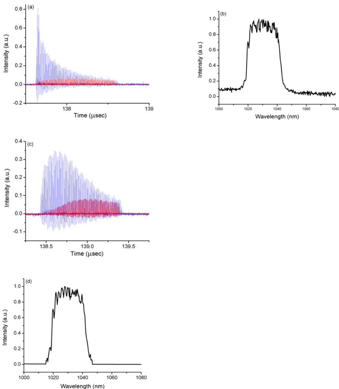
Fig. 12. Output (blue line) - Input (red line) pulse trains ((a) and (c)), and corresponding output spectra ((b) and (d)), respectively, for two different 1- $\mu$ s signal bursts at a repetition rate of 1 kHz.
