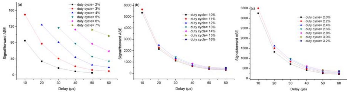
Fig. 6. The measured signal-to-ASE power ratio for pulse burst lengths of (a) 20  $\mu\text{s}$ , (b) 100  $\mu\text{s}$  at 1 kHz and (c) 100  $\mu\text{s}$  at 200 Hz as a function of the delay between the rising edges of the pump and signal emissions for various pump duty cycles. The lines are only to guide the eye.
