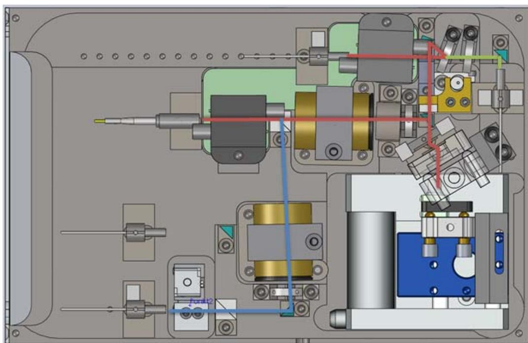
Fig. 6. Laserbox-Design of the 500 MHz oscillator. Basically the same optics as in the breadboard-setup are used, although due to better mechanical properties the cavity can be even more compact with a free-space optical length of only 25 cm.
