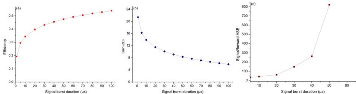
Fig. 8. The measured (a) pump-to-signal conversion efficiency, (b) signal gain factor and (c) ASE formation as a function of signal burst duration for a 100- $\mu\text{s}$  pump pulse at a repetition rate of 1 kHz. The lines are only to guide the eye.
