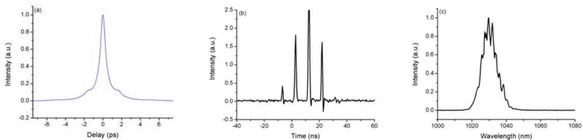
Fig. 14. (a) Autocorrelation result, (b) output pulse train per pick which was repeated at 10 kHz (c) output spectrum for the amplified pulses of 20 μJ average energy that were compressed to 500 fs.
