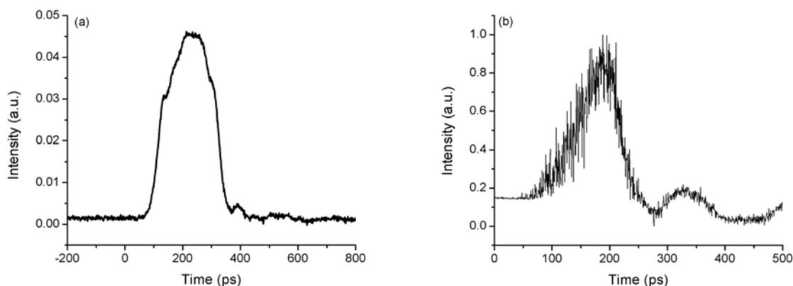
Fig. 3. Measured pulse duration (a) after the 210-m stretch fiber at full repetition rate of 104 MHz and (b) after the second preamplifier for a signal burst of 1  $\mu$ s at 1 kHz, 130  $\mu$ s pump pulse. The noise in (b) is due to the low repetition rate of 1 kHz.
