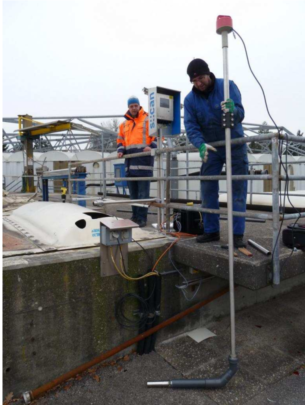
Figure 33: UV/VIS spectrometer fixed rigidly at the end of a metal bar in the inflow channel to the primary clarifiers of Linz WWTP
