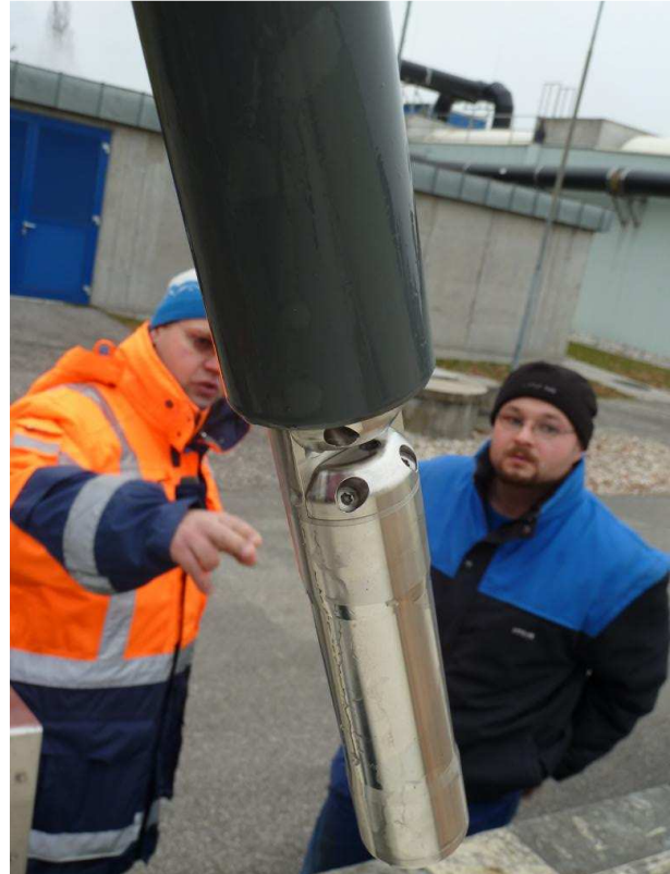
Figure 33: UV/VIS spectrometer fixed rigidly at the end of a metal bar in the inflow channel to the primary clarifiers of Linz WWTP
