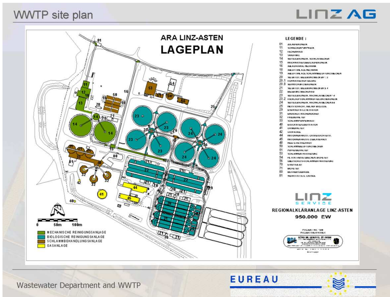
Figure 27: Map of WWTP Linz with the two primary clarifiers in green and indicated with No. 14
