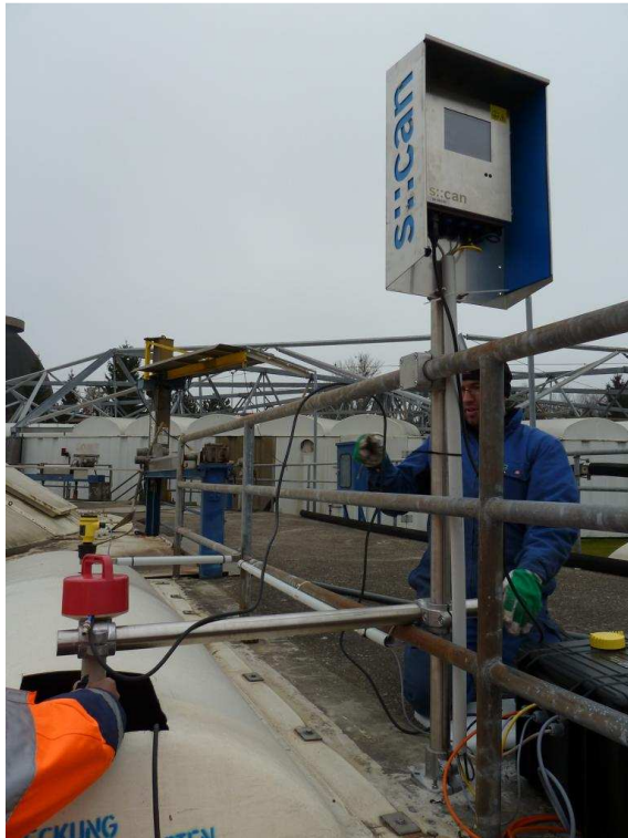
Figure 31 Inflow measurement site with the installed UV/VIS spectrometer, the ultrasonic probe and the industrial PC for data recording.
