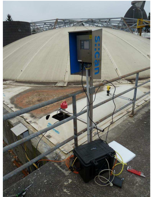
Figure 31 Inflow measurement site with the installed UV/VIS spectrometer, the ultrasonic probe and the industrial PC for data recording.
