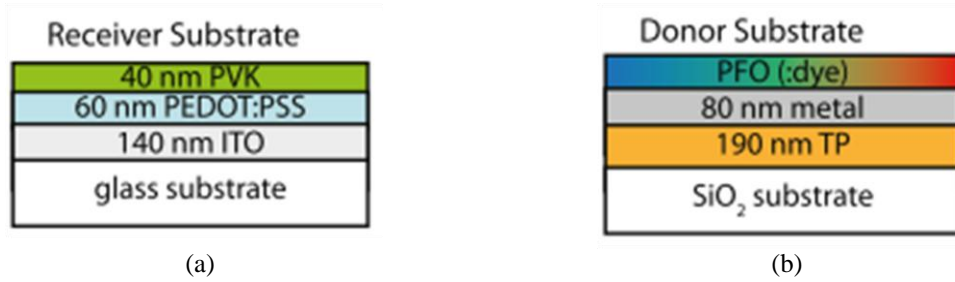
Figure 10: Structures of the receiver (a) and the donor (b) substrates
