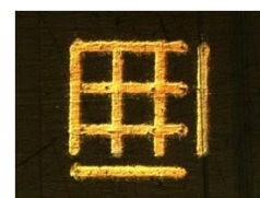
40 \mu\text{m} wide LIFT-printed silver lines on PET
