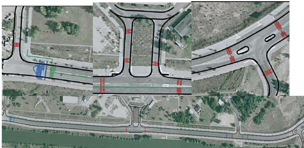
Figure 19: Red: loops, blue: radar, green: already decomposed temperature sensors
