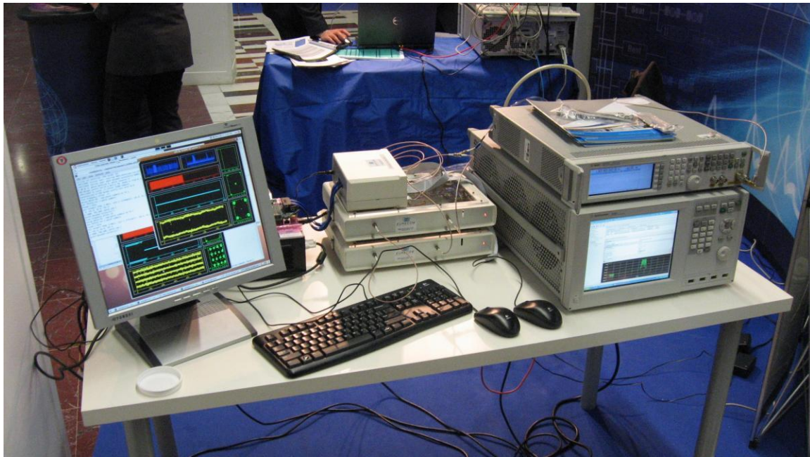
Figure 5-3: Demonstration setup of OpenAirInterface Express MIMO platform and Agilent PXB.
