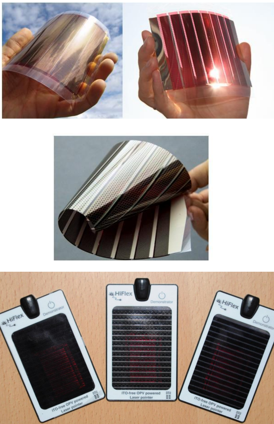
Figure 1 Pictures of S2S processed (Top) and R2R processed ITO free modules (middle) and three variants of ITO free powered laserpointer demonstrators
