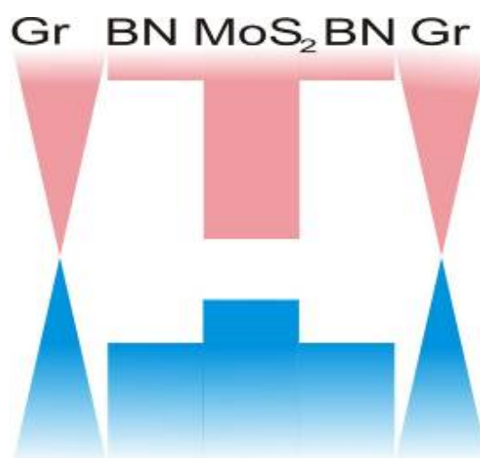
Figure 19: Gr/BN/MoS 2 /BN/Gr structure: blue is the valence band and pink is the conduction band [32].
