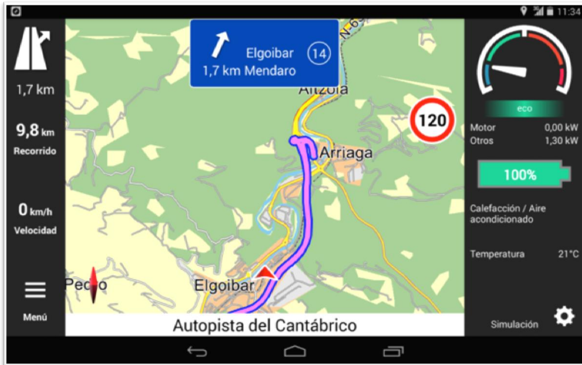
Figure 4.2.2.18 Navigation instructions and DoD estimation on PTV Navigator
