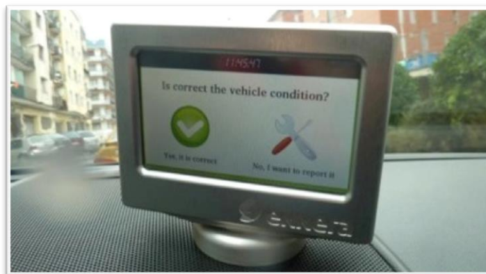
Figure 4.2.2.8 Vehicle condition verification by OBU
