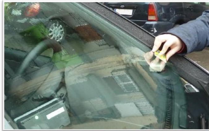
Figure 4.2.2.7 Picking up the vehicle. RFID user card read through windscreen
