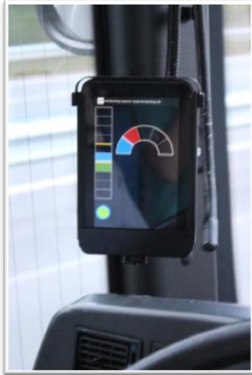
Figure 7.1.2.3 HMI giving instructions to the driver
