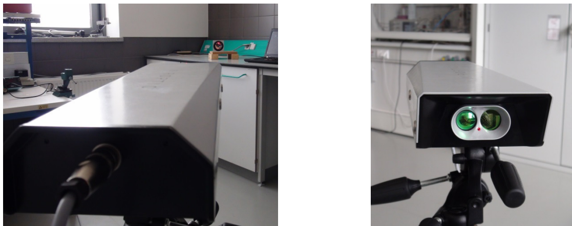
Fig. 15 The fully operational formaldehyde sensor. The retro-reflector that defines the measurement path is shown in the background
