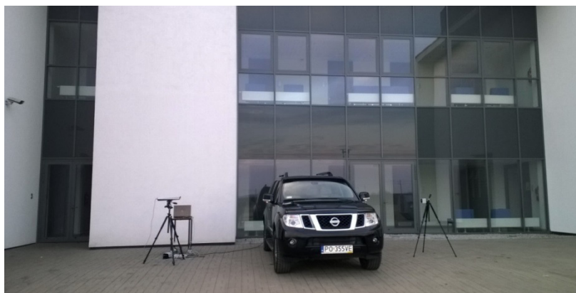
Fig. 4.20 Validation test utilizing a Nissan SUV. 106 ppm of alcohol vapour is generated in the passenger compartment utilizing a Breath Test Simulator
