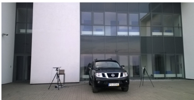
Fig. 4 The laser based sensor system of WideLase for remote detection of alcohol against drunk driving.
