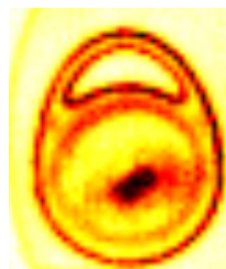
Figure 24 The image of an RFID key has been taken using the 180 GHz and the 220 GHz harmonic generated by the Aleph TX v. 0.3. the images reveal the internal structure of the key as it is clear comparing them with the visible image (top left) of the unpackaged key.
