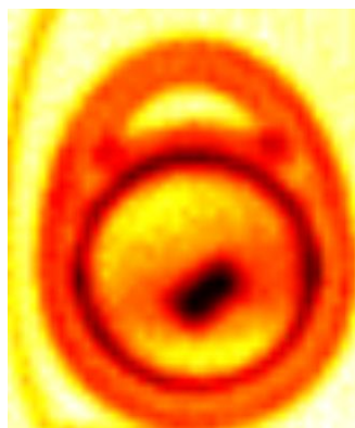
Figure 24 The image of an RFID key has been taken using the 180 GHz and the 220 GHz harmonic generated by the Aleph TX v. 0.3. the images reveal the internal structure of the key as it is clear comparing them with the visible image (top left) of the unpackaged key.
