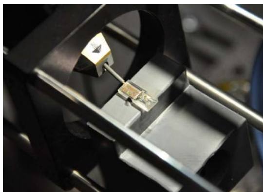
Figure 23 The Aleph THz transmitter (left) and a detail of the whole measurement setup.
