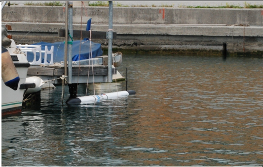
Figure 9: Folaga 1 (F1) moored to the pier. In this configuration the Folaga had the acoustic interface in the water for communication with Folaga 2 (F2) and the wireless antenna always out of the water to communicate with the UAN Gateway and hence with the Command and Control.
