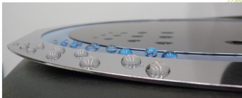
Figure 1: Calibrated droplets on various wafers /materials for frame and tape for experimental drying tests
