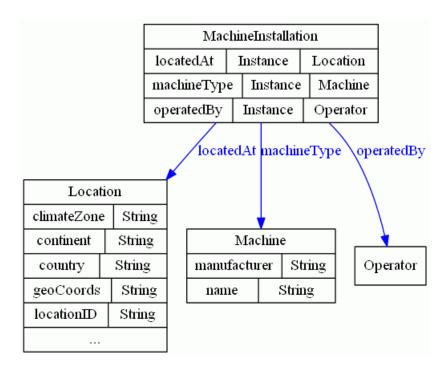
A machine model (class *Machine*) has a *manufacturer* and a *name*. Each machine installation (class *MachineInstallation*) has a particular machine model (relationship *machineType*), a location (relationship *locatedAt* to class *Location*), and is operated by some responsible operator (relationship *operatedBy* to class *Operator*).
