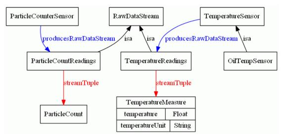
Analogously a **temperature sensor** (*TemperatureSensor*) measures the current temperature of some artifact. It produces a raw data stream of **temperature readings** (*TemperatureReadings*), which is a stream of **temperature measurements** (*TemperatureMeasure*). A temperature measurement has attributes *temperature* and *temperatureUnit* (Celsius, Fahrenheit, Kelvin).
