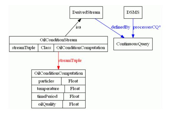
A tuple in the oil condition stream contains a value estimating the oil quality based on the temperature readings and particle counts during a time period. The values are computed as a continuous query (relationship *definedBy*) based on two other raw data streams, a particle count stream and a temperature reading stream. To enable explaining the estimated value of
