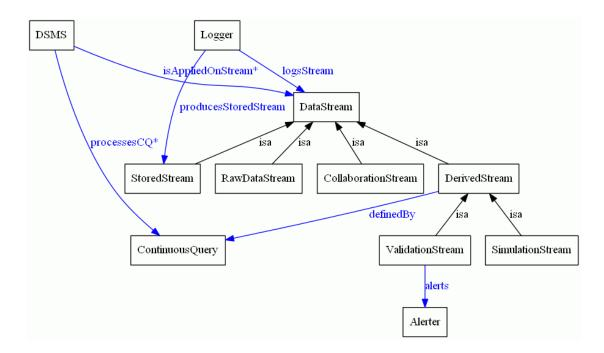
A **DSMS** produces one or several **derived streams** defined by a continuous query (relationship *definedBy*). If desirable and feasible any kind of data stream may be continuously saved on disk (class *StoredStream*) by running a **logger** (relationship *logsStream*). The output of a validation stream can be fed into an **alerter** (relationship *alerts*), which is a program notifying users and systems that some unexpected behavior has occurred.
