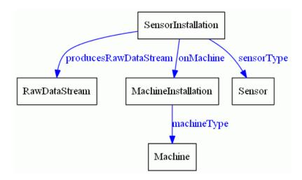
The class *SensorInstallation* represents **sensors** installed in a particular **machine** (class *MachineInstallation* and relationship *onMachine*). Each sensor is of a particular kind (class *Sensor* and relationship *sensorType*). A machine is also of a particular kind (class *Machine* and relationship *machineType*). A sensor produces a **raw data stream** (class *RawDataStream* and relationship *producesRawDataStream*).
