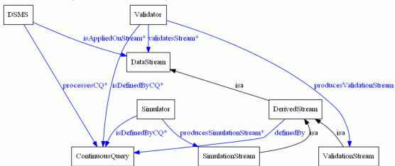
A **DSMS** processes a number of **continuous queries** (relationship *processesCQ*). A continuous query (CQ) is an expression executed by a DSMS, which defines how the DSMS
