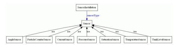
The particular kinds of sensors used by Hägglunds are subclasses of type *Sensor*. The different kinds of sensors will be further specialized by subclassing each specific sensor class. Thus, all kinds of sensors used by Hägglunds are modeled by this RDF-Schema view:
