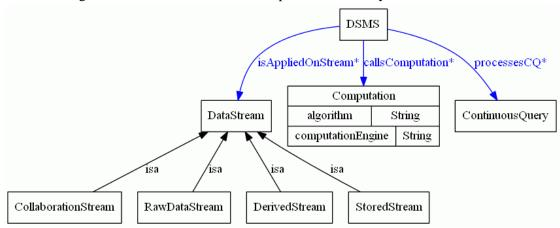
Continuous queries may involve different kinds of **computations** over streams. The computations are called as plug-ins to the DSMS (relationship *callsComputation*). A computation implements some algorithm (attribute *algorithm*) by calling some computation engine (attribute *computationEngine*). For example, a simulation stream may be expressed as a continuous query executing some computation algorithm executed by a Python engine.
