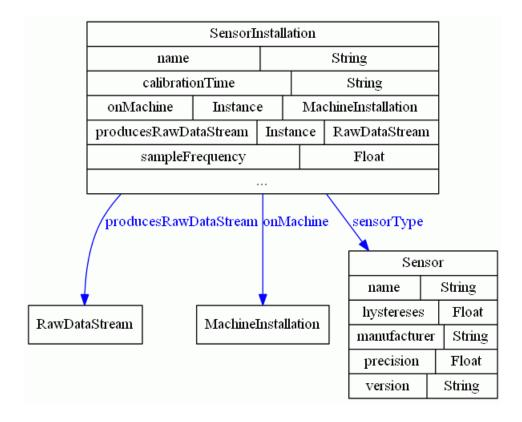
Each **sensor model** (class *Sensor*) has the attributes *name*, *hysteresis* (its reaction time), a *manufacturer*, *precision* (of the values it measures), and a *version*.
