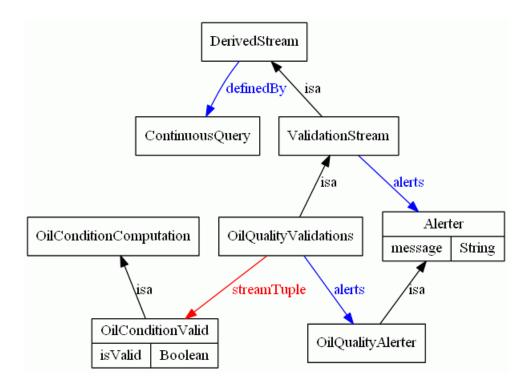
A validation stream detecting oil quality validations, *OilQualityValidations*, is defined by a continuous query that produces tuples of class *OilConditionValid*, which extends the derived stream *OilConditionComputation* with a flag *isValid* indicating whether or not the oil quality is satisfactory. If the oil is not of satisfactory quality an alerter is invoked that sends a message to the responsible operator.
