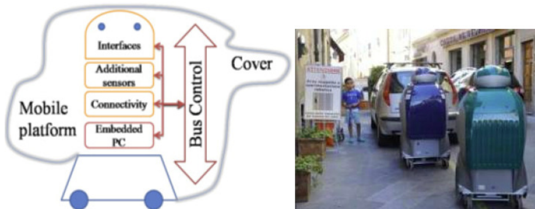
Figure 5 High level overview of the main components integrated in the outdoor robotic platform (left). The DustCart robotic platforms provided by RT (right)
