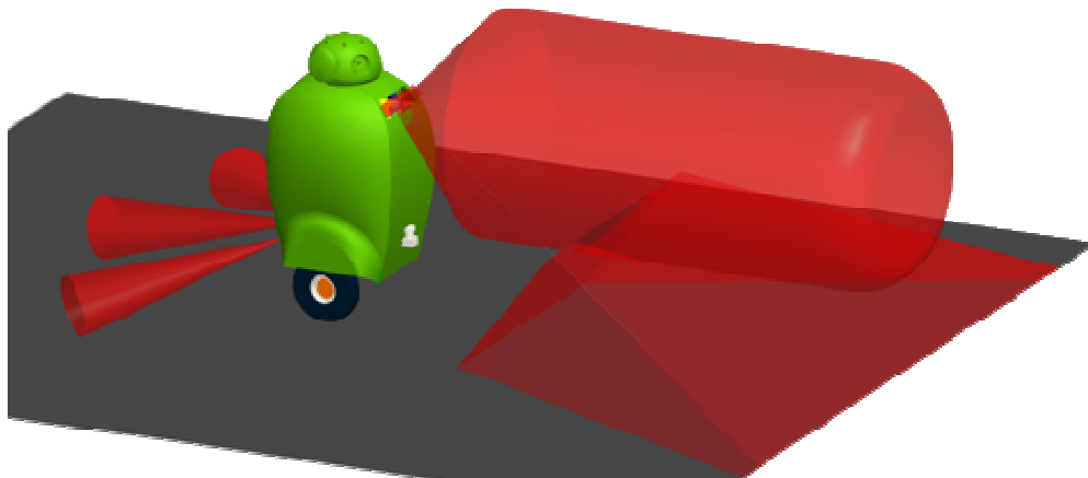
Figure 6. The obstacle detection sensors and their detection space.
