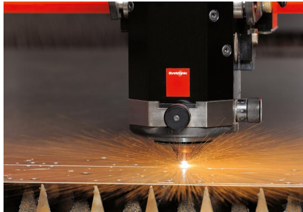
Laser cutting head in action
