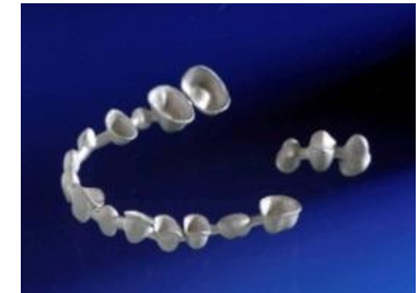
Examples of parts made by selective laser melting
