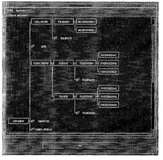
5. The geometry is selected and *attackmeirfs* are defined. Attachments are named 'faces' on the component which can be used to orientate and attach the component to other components in an assembly.
