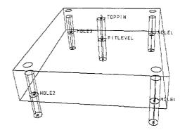
6. The components parameters (attributes which alter the geometry) are derived automatically from the geometry. Extra attributes can then be added manually. Tolerances can be associated with any attribute (+/- or limit and fit codes).
