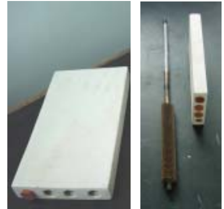
17. Ceramic Evaporator with Heat Pipe
