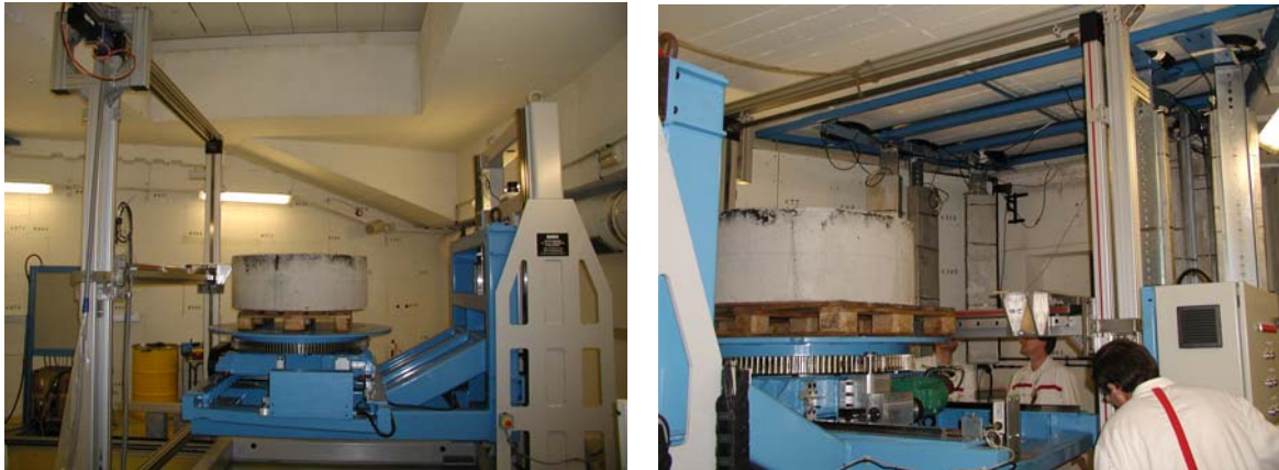
Figure 2.4.2 Experimental set-up of the third in situ validation test at the Saphir linear accelerator location of CEA Saclay, France. The concrete mock-up is situated at the conveyor, while the instruments will be placed on the platform of the 3Drise system (see also Figure 2.4.3), so that can be positioned and exactly adjusted behind the mock-up.
