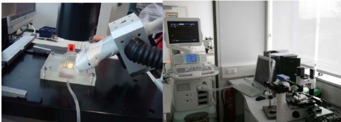
Experimental setup for in-vitro study (flow phantom attached to the microscope, ultrasound probe held in place with a stativ)..
